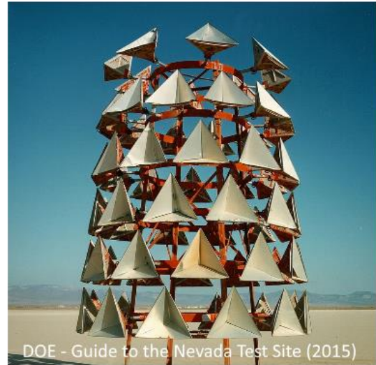
Figure 20. (Left) Illustration of parallel reflection via triple orthogonal redirection. (Right) Array of corner retroreflectors at the Nevada Test Site.
