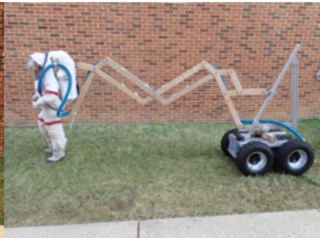
Figure 21: Passive pantographic umbilical handling mechanism
