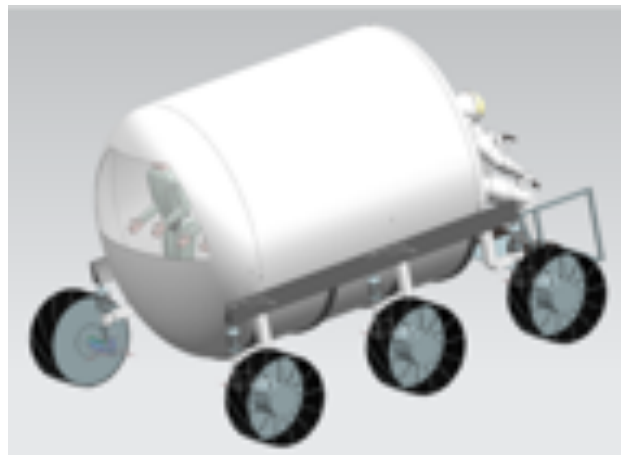
Figure 7: BioBot configuration (f) — pressurized two-crew transport
