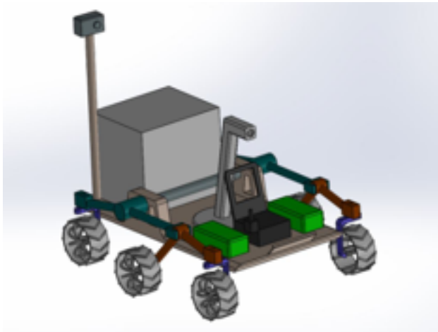
Figure 2: BioBot configuration (a) — transport of life support hardware only [The CAD image shows a four-wheeled rover with a simple representation of two robot arms for manipulating the astronaut's umbilical.]
