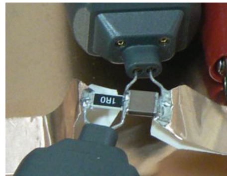
Fig. 9 Chip capacitor-chip resistor arrangement.
