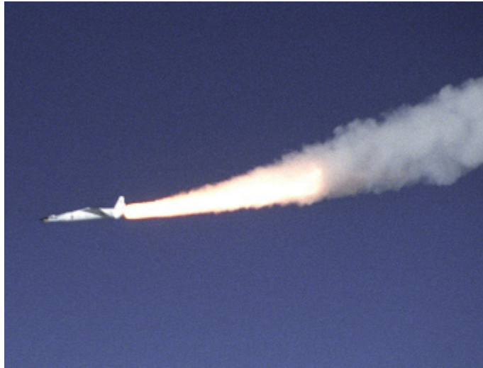
Figure 4.7-13: The third X-43A accelerates to Mach 9.7 Prior to release from its Pegasus Booster, 16 November 2004, following air-launch over the Pacific Ocean from its Boeing NB-52B mother ship. NASA Image EC04-0325-37.
