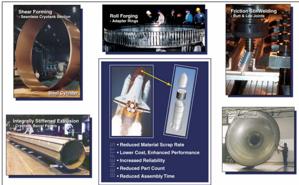
Figure 4.9-6: Near-Net-Shape Manufacturing of Al & Al-Li Alloys For Launch Vehicle Structures.
