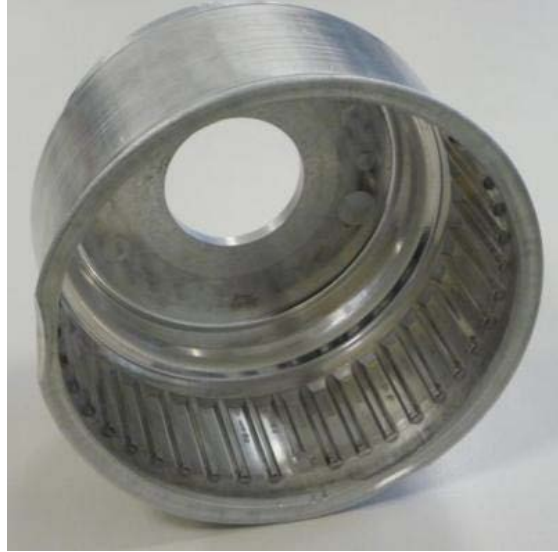
Figure 6.2-12: As-Formed, 0.3 m Diameter Al-Li 2195 Alloy Part. 16
