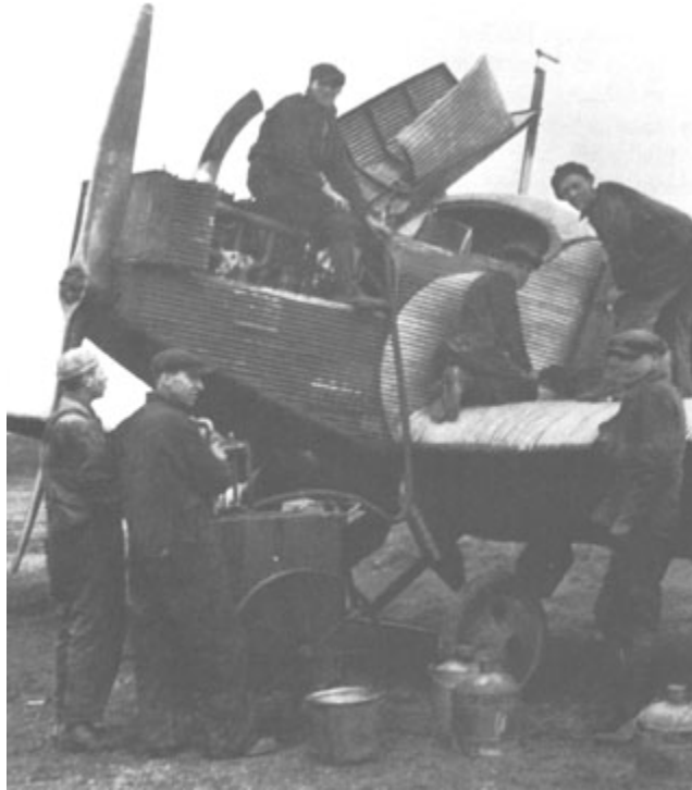
Figure 3.1-2: The Junkers J.L. 6 was probably the earliest all-metal plane, built in Germany in 1919 as the F 13 and imported to the United States by John Larsen to be used as a mail plane.
