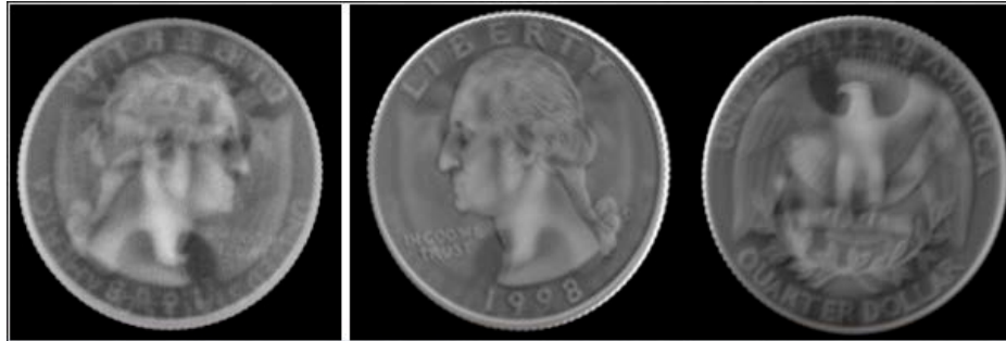
Figure 13.2-10: X-ray Images Showing Conventional (Left) and Laminography with Reverse Geometry X-ray (Center and Right) Capabilities. Note that the laminography can produce slice images similar to CT. [Image is from Digiray®.]
