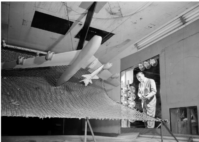
Figure 3.4-1: A one-twentieth scale model of the X-15, originally suspended beneath the wing of a B-52 was tested in the Langley High-Speed 7 × 10 Foot Tunnel, Around 1957. http://www.archive.org/details/GPN-2000-001882 .
