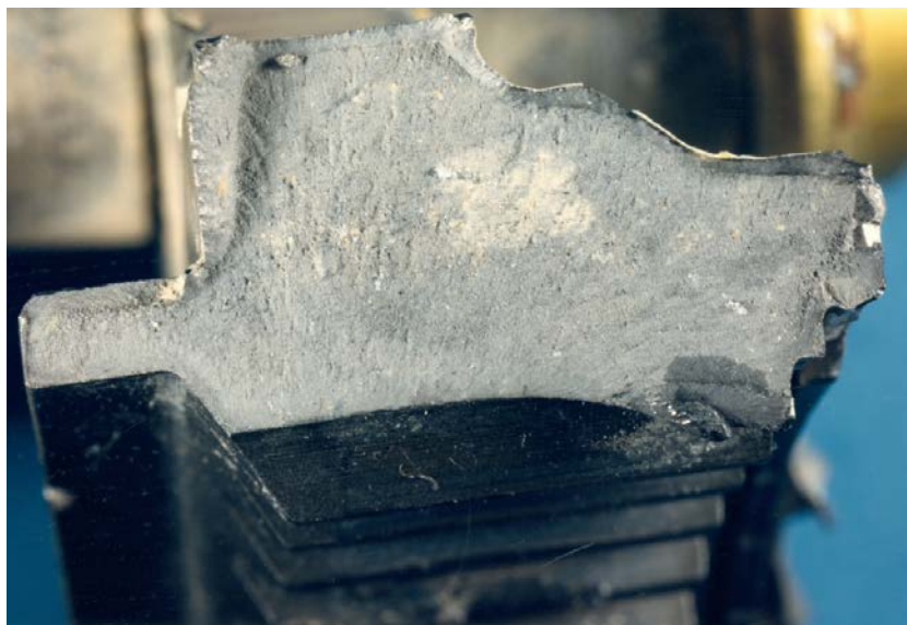
Figure 2.10-4: Typical Fracture Surface of Transmission Ring Gear.
