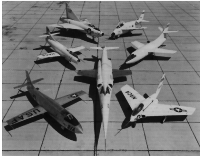
Figure 4.6-2: Typical high-speed research aircraft that made headlines in the 1950s. The Bell X-1A (lower left) had much the same configuration as the earlier X-1. Joining the X-1A were (clockwise); the Douglas D558-I Skystreak; Convair XF92-A, Bell X-5 with variable sweepback wings, Douglas D-558-I Skyrocket; Northrop X-4; and (Center) the Douglas X-3.
