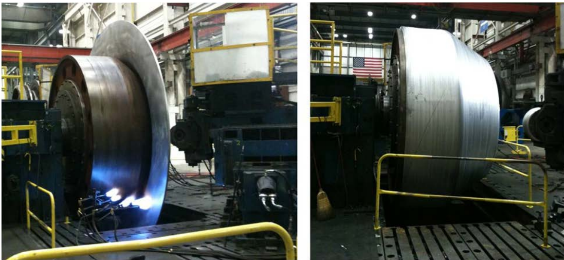
Figure 4.9-21: Spin Forming The Single-Piece MPCV Forward Pressure Vessel Bulkhead.
