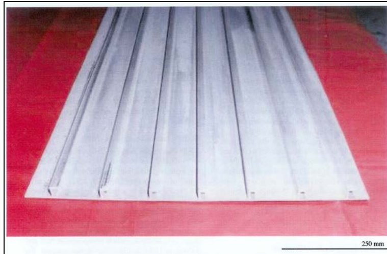
Figure 6.2-2: Extruded 2090 Integrally Stiffened Panel. 4
