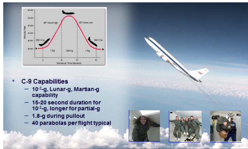
Figure 6.3-6: Microgravity Testing aboard JSC's C-9 Aircraft.
