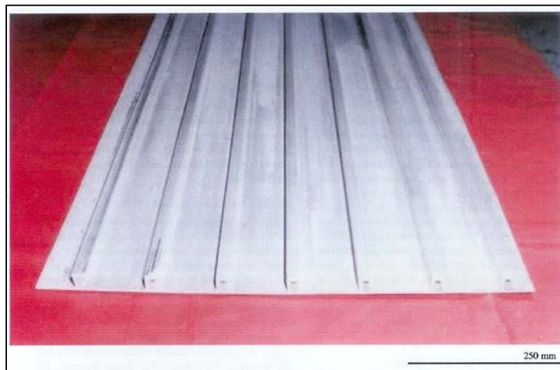
Figure 16.7-1: Extruded 2090 Integrally Stiffened Panel.
