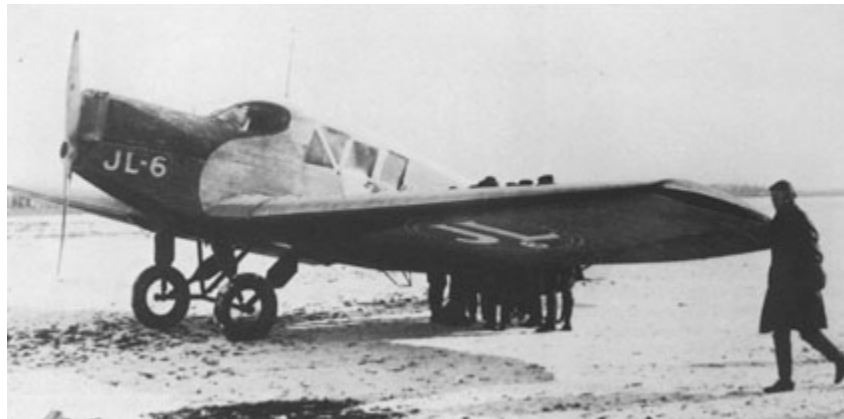
Figure 3.1-1: The Junkers J.L. 6 represents an important step forward in technology. It was probably the first plane with the fuselage, wings, and skin all constructed of metal.
