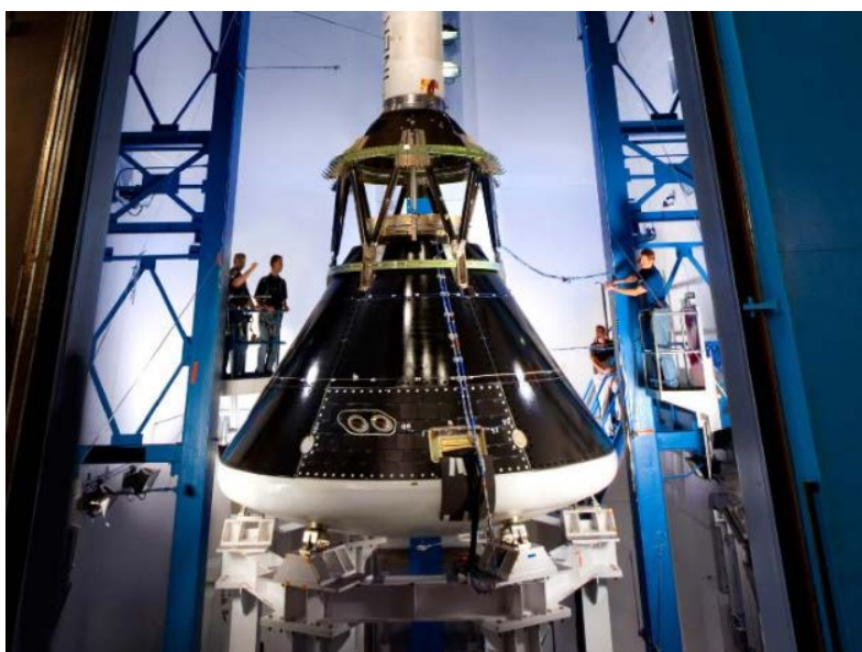
Figure 1.2-7: Orion MPCV, or Multi-Purpose Crew Vehicle, and LAS, or Launch Abort System, test craft in the acoustic chamber at Lockheed Martin's facilities near Denver.
