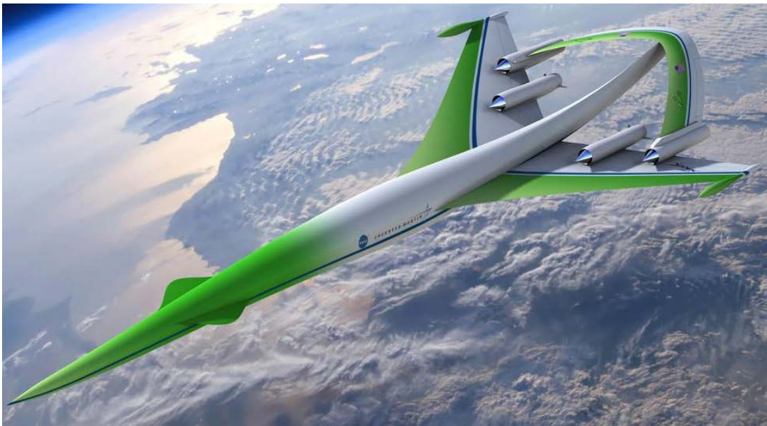
Figure 4.6-13: Future Aircraft Design for Supersonic Flight Over Land. Concept is an “Inverted-V” engine under wing Configuration.
