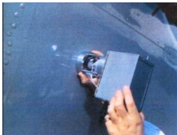
Figure 13.2-8: Electromagnetic Flux Nulling Probe Inspecting an area near a lap joint on an aircraft.
