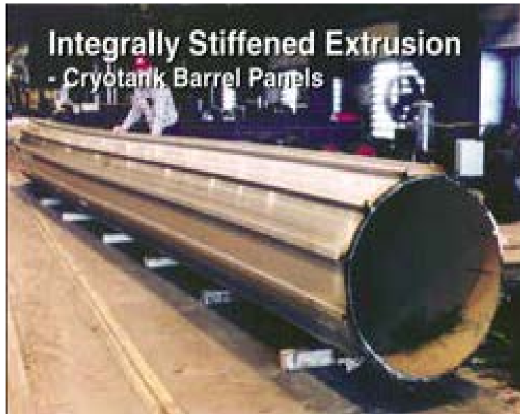
Figure 6.2-3: Extrusion of an Integrally Stiffened Barrel Section for Cryotanks.
