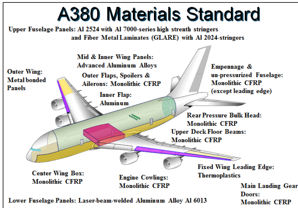
Figure 2.1-4: Materials Used in Airbus A380. 4
