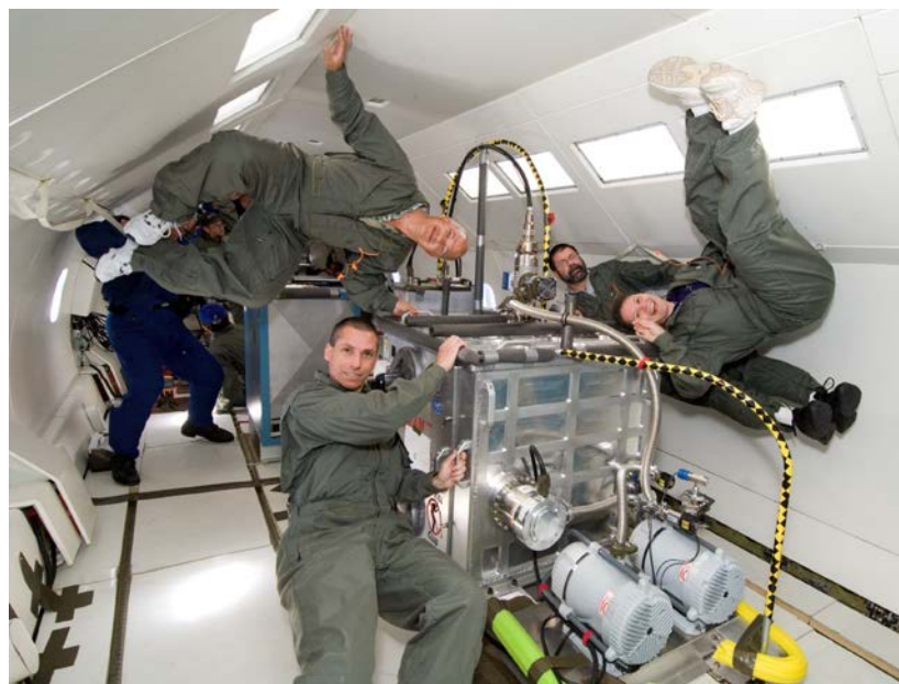
Figure 6.3-7: Testing the EBF 3 Portable System Aboard the NASA JSC C-9 Aircraft.
