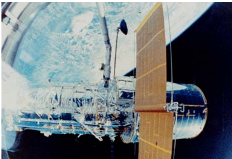
Figure 5.7-3: The P100/6061 Al High-Gain Antenna Wave Guides/Boom for the Hubble Space Telescope (HST) Shown on the HST as it is Deployed in Low-earth Orbit from the Space Shuttle Orbiter.
