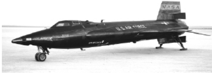
Figure 4.7-1: North American X-15 Mach 6+ Hypersonic Trans-Atmospheric Research Aircraft. NASA Image E-7411.
