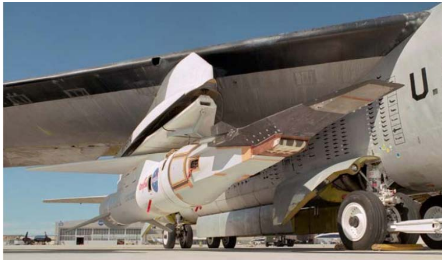
Figure 2.5-1: Hyper-X experimental aircraft mounted under the wing of a B-52B airplane, ready to be carried to test altitude.
