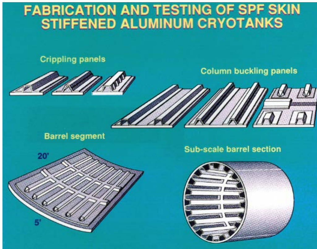
Figure 4.9-9: Fabrication and Testing of SPF Stiffened Aluminum Cryotanks.
