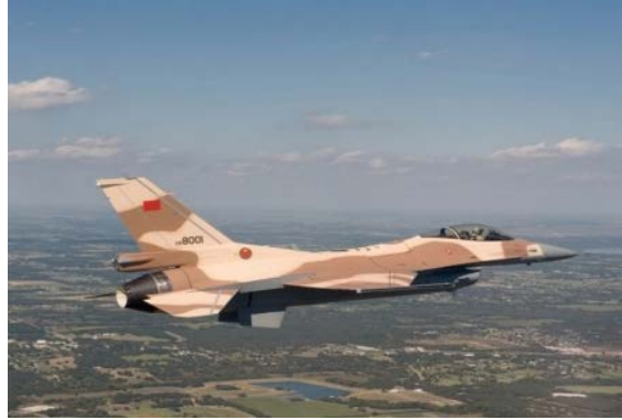
Figure 5.4-5: The Al-Li alloy 2098, developed under the NASA-sponsored High-Temperature Aluminum Alloy Program is used in the F16 Fighter Aircraft.
