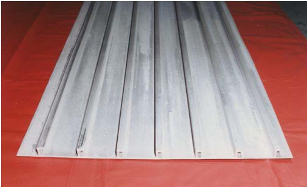
Figure 5.3-3: Extruded 2090 Panel in As-Received Condition.
