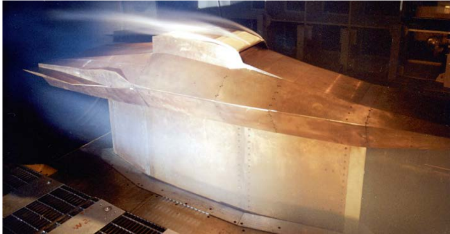
Figure 4.7-11: Wind tunnel tests were a necessary step before the first flight attempt, as in this Mach 7 test of a full-scale model with spare flight engine in Langley's 8-Foot High-Temperature Tunnel.
