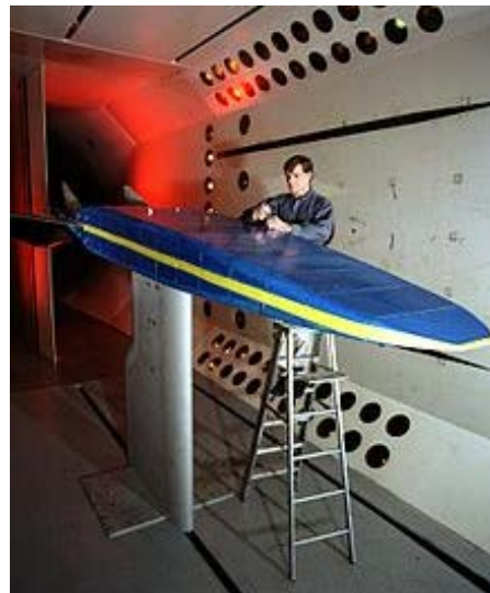
Figure 5.8-2: X-30 Model in a Wind Tunnel.
