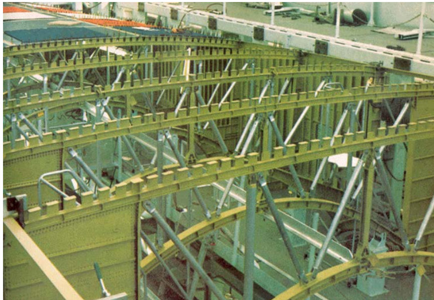
Figure 5.7-1: Mid-Fuselage Structure of Space Shuttle Orbiter Showing Boron-Aluminum Tubes. (Photo courtesy of U.S. Air Force/NASA). http://www.tms.org/pubs/journals/JOM/0104/Rawal-0104.html .
