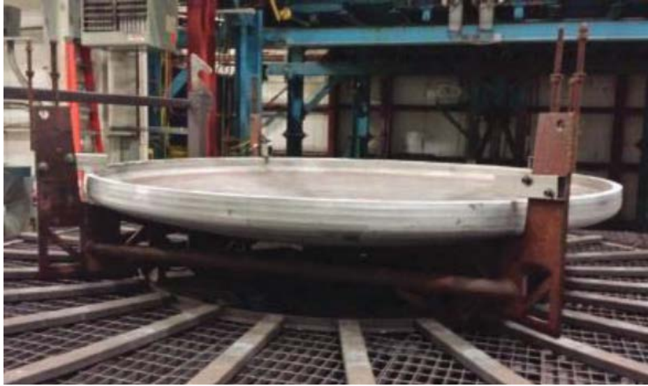
Figure 15.7-6: Aft Bulkhead Following Heat Treatment.
