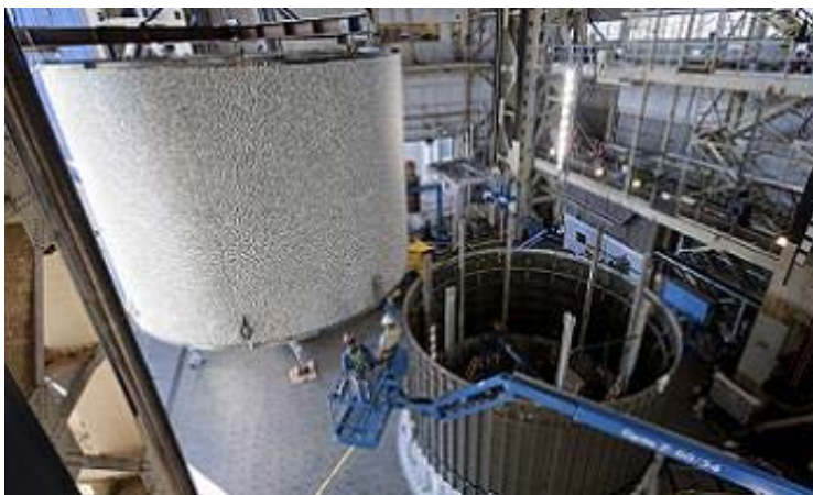
Figure 2.8-2: “External-Tank-like Test Article,” 8.4 m in diameter and 6.1 m tall, tested at NASA Langley Research Center.
