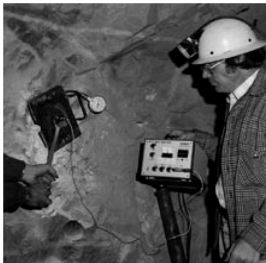
Figure 13.2-1: Heyman Shown in a Bureau of Mines Test of the Bolt Monitor for a Mine Bolt.
