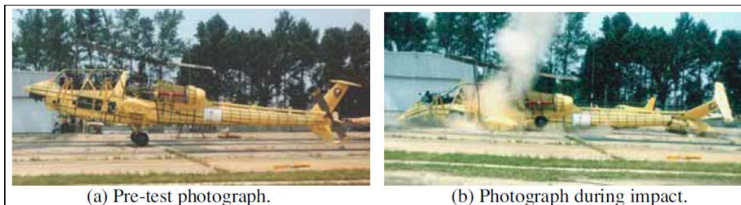
Figure 4.5-3: Pre- and Post-Test Photographs of the Bell YAH-63 Helicopter.
