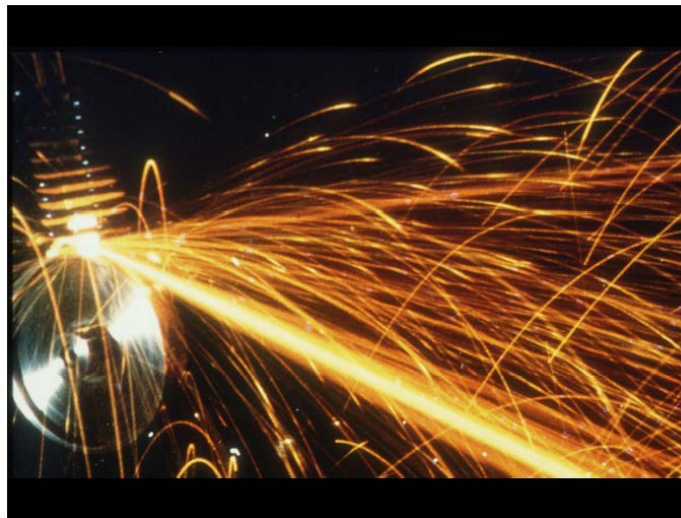
Figure 15.1-6: Melt Spinning to Produce Metallic Glass.
