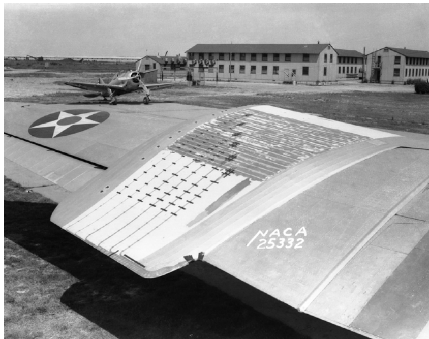
Figure 6.5-1: In the spring of 1941 Langley installed an experimental low-drag test panel on the wing of a Douglas B-18 airplane. The panel was fitted with suction slots and pressure tubes for a free flight investigation of the transition from laminar to turbulent flow in the boundary layer. The pressure at each tube was measured by liquid manometers installed in the fuselage. http://www.archive.org/details/GPN-2000-001244 .
