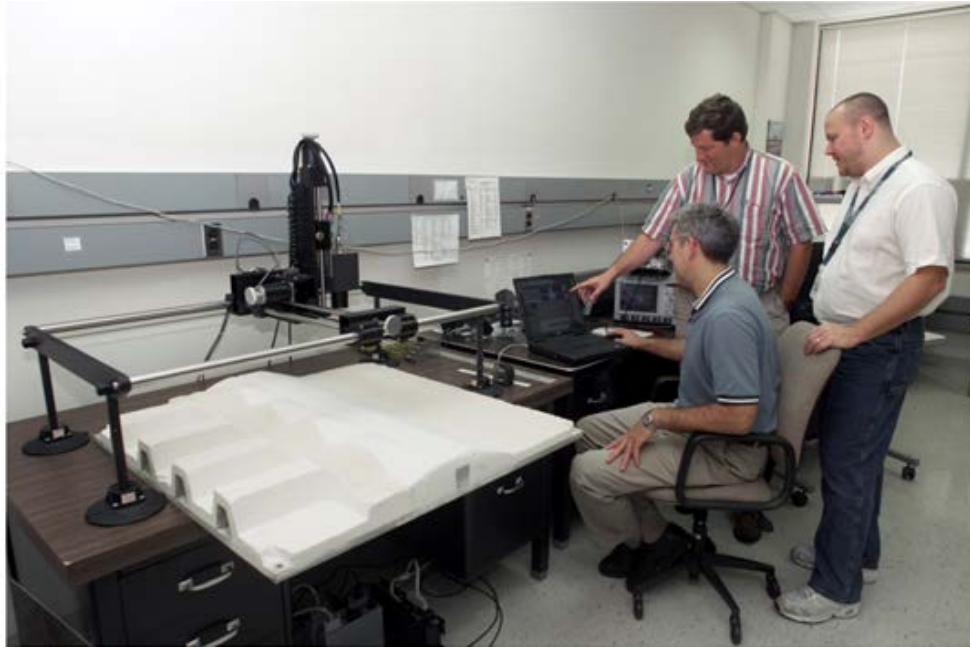
Figure 13.2-14: Research on T-Ray System at NESB for Application to Shuttle External Tank Foam Inspection.
