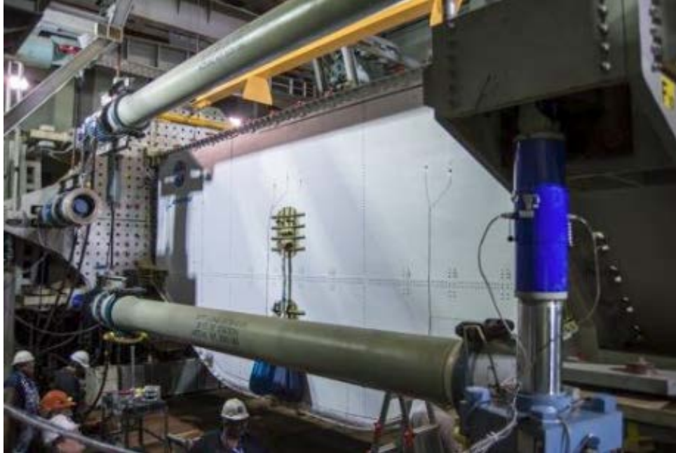
Figure 9.5-2: Multi-Bay Box Located Between Platens.
