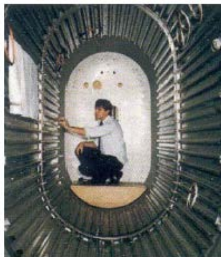
Figure 4.7-3: Fuselage Section of National Aerospace Plane (NASP), SiC/Ti Stiffeners, Spot-Welded to 4' × 4' Panels.
