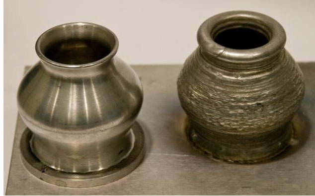
Figure 16.8-3: Electron Beam Freeform Fabrication (EBF 3 ); As-deposited and Machined.
