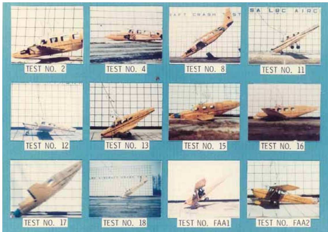
Figure 2.2-3: Photographs of Several GA Aircraft Full-Scale Crash Tests Performed at the IDRFB.
