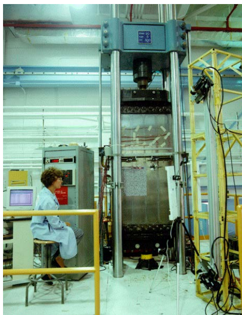
Figure 8.11-2: Wide Stiffened Panel in Test Frame at NASA LaRC.
