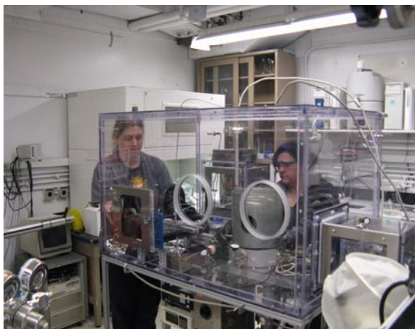
Figure 6. The O/OREOS sample-fabrication-and-test facility for the flight sample cells at NASA Ames. Contained within a glove-box, this high-vacuum thin-film deposition system includes an Ocean Optics HR400CG-UV-VIS spectrometer (200 - 1100 nm) for film characterization.
