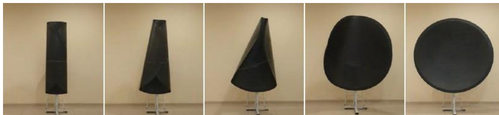
Figure 8. Deployment of the self-deployable shell reflector (duration: 1.4 s) 13
