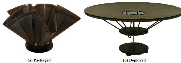
Figure 7. Flexible precision reflector before and after deployment 11
