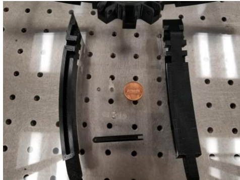
Figure 7. 3D printed and moving parts of the radial folding deployment mechanism (a penny is used for scaling purposes).
