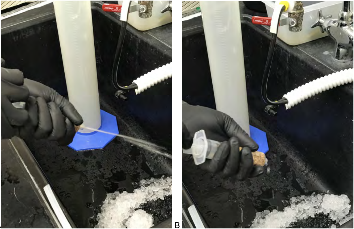
Figure 17. Pressure applied to the syringe (A) and mycelium lost in the process (B).
