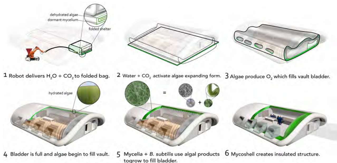
Figure 2. Fully encased structure self assembles when water, CO 2 and heat are added by robots.
