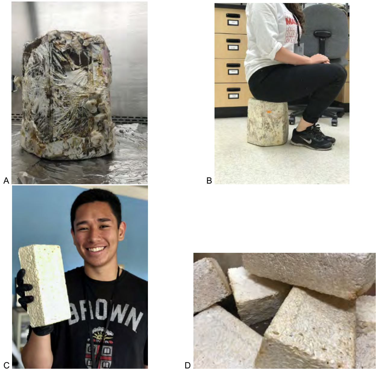
Figure 7. A, stool after 2 weeks of growth, prior to being baked. B, iGEM team member Emilia Mann sitting on the stool after it has been baked. C, iGEM team member Javier Syquia holding the first brick produced by the team. D, pile of bricks produced with mycelium and yard waste, wood chips.
