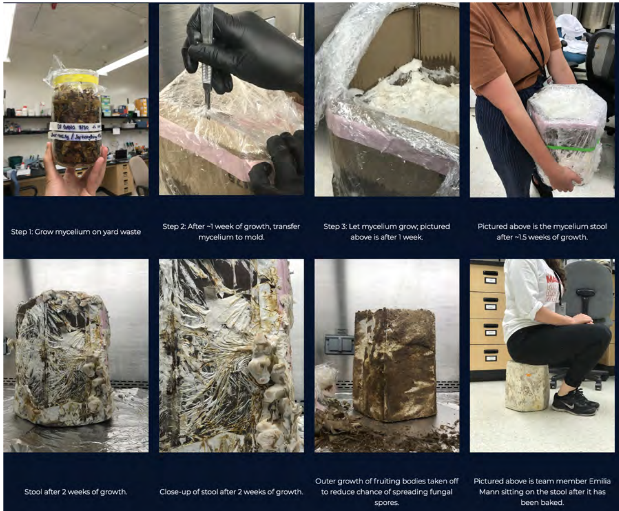
Figure 46. Production process including crafting, baking, and testing the stool. http://2018.igem.org/Team:Stanford-Brown-RISD/Human Practices
