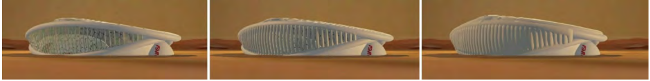
Figure 31. Extra radiation shield can be deployed through hydrogen bladders when solar wind is forecasted.
