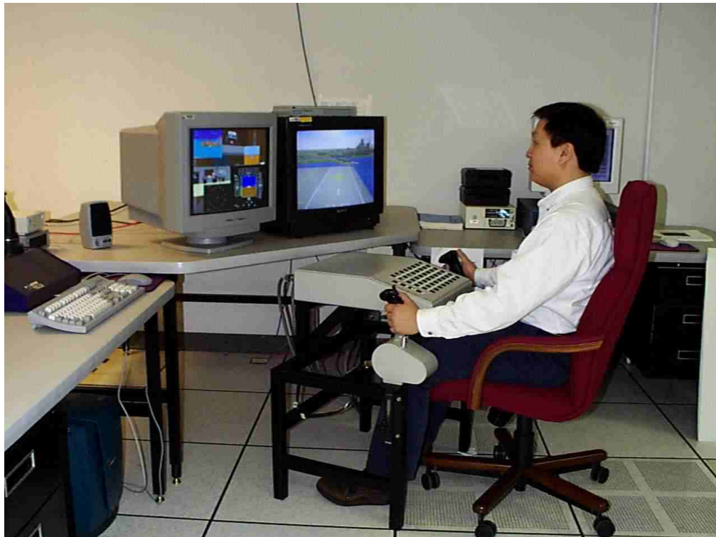
Figure 6.2. Desk-top development simulation work station.
