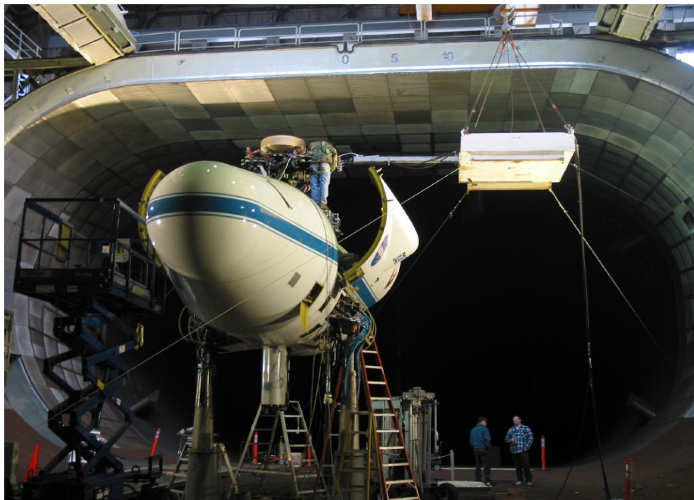
Figure 5.18. Dynamic calibration setup for LRTA in the NFAC.
