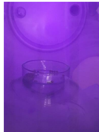
Figure 10 : Radish seedlings in a sub-atmospheric plasma treatment.
