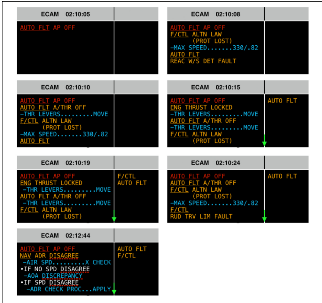
Figure 5. Air France 447 ECAM displays if no messages had been erased (BEA, 2012, pg. 97).
