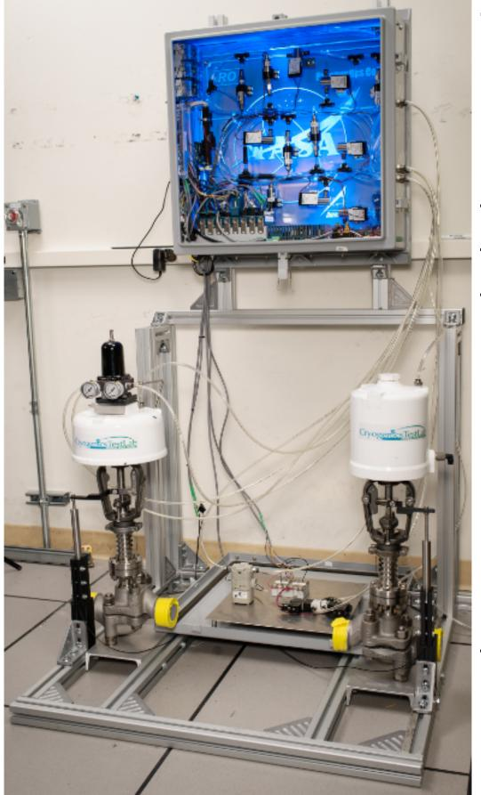
The Cryogenic valve testbed injects controlled faults into the cryogenic fuel valve system in order to accurately determine failure behavior. Data obtained from such experiments is useful development the tor algorithms determining remaining useful life and end of life for the valves in the fuel loading system. Additionally, the diagnostic and prognostic methods developed with this system can potentially be used for future missions to help manage safety or degradation in a similar system.
