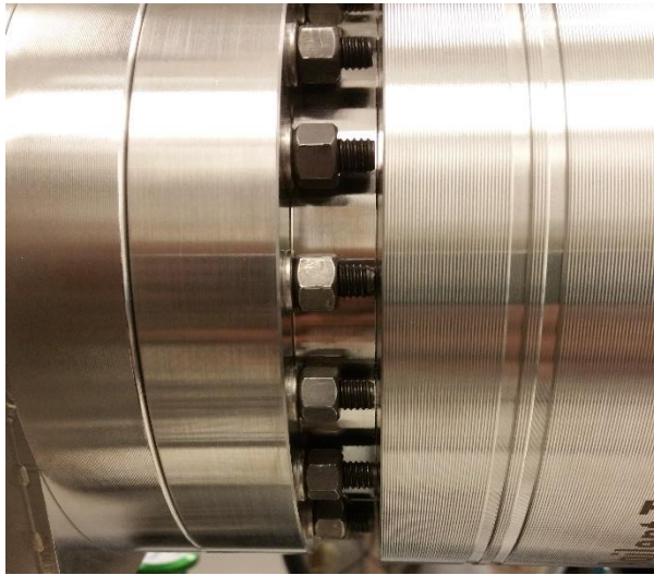
Figure 1: Current setup of turbo-molecular pump with installed rods. One of the issues while installment was the difficulty to install the rods given the small clearance to insert and tighten the nuts.
