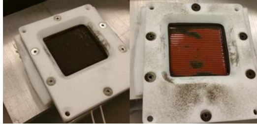
Figure 3: Before and after clearing dust while the HVPS had the faulty connection.
