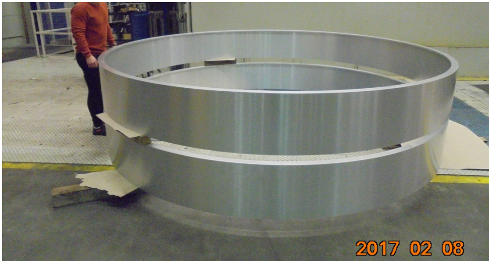
Figure 4. Two ISC ring preforms as delivered to MT Aerospace. (Image used with permission from MT Aerospace)
