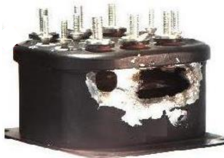
Failed relay due to tin vapor arcing
