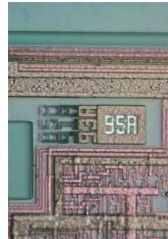
Optical images of a decapsulated part
