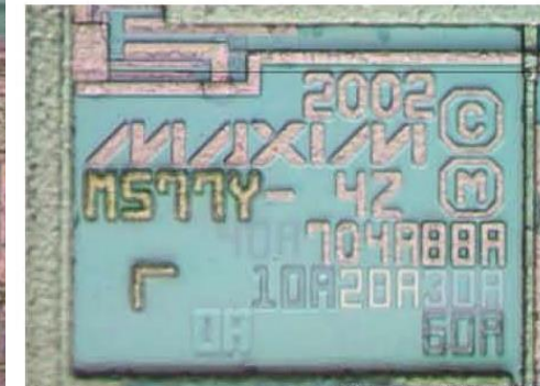
Optical images of a decapsulated part
