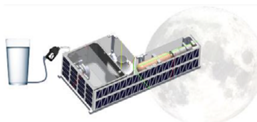
Cislunar Explorers 6U-sized CubeSat splits into two; each uses water for its propellant.
