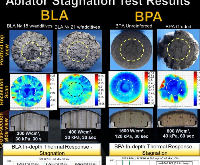
Higher density formula with additives shown to result in lowest bondline temperature
