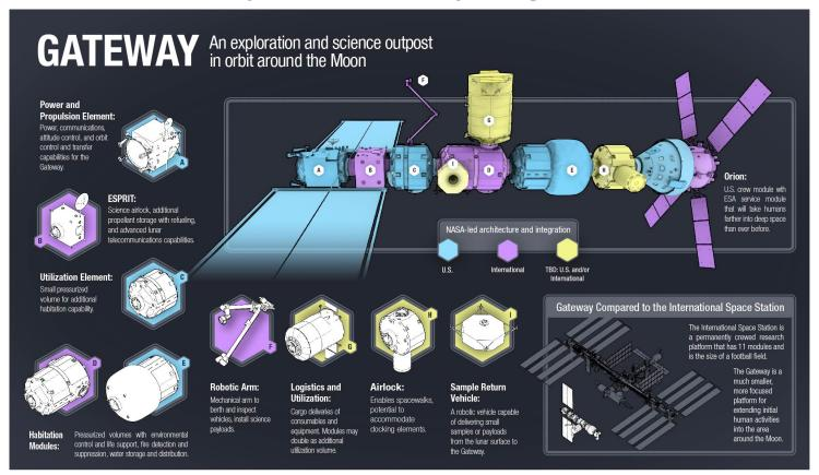
Lunar Orbit space station is intended to serve as an all-in-one solar-powered communications hub, science laboratory, short-term habitation module, and holding area for rovers and other robots.
