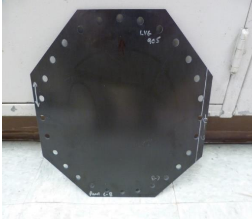
Figure 10. T800/F3900 panel used for impact testing.
