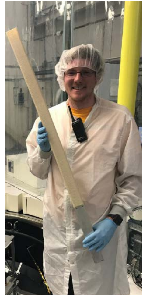
MIS Mechanical Engineer Deejay Riley with 850 mm Beam printed in a TVAC chamber
