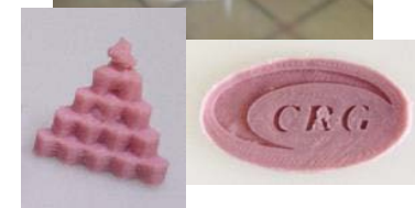
FDM prints using reclaimed anti-static bagging film with reversible cross-linking additive (image from CRG)
