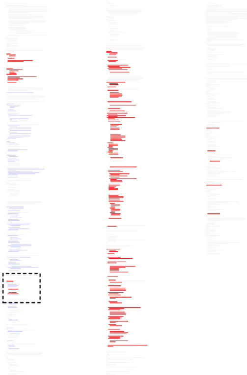
Fig. 14. Decluvi's file view for the file util.c of program bc. Each line of pixels correspond to one source code line. Blue (medium gray in black and white) represents lines with vertices belonging to the 2nd largest cluster and red (dark gray) represents lines with vertices belonging to the largest cluster. The rectangle marks function init_gen , part of both clusters. (For interpretation of the references to color in this figure legend, the reader is referred to the web version of the article.)
