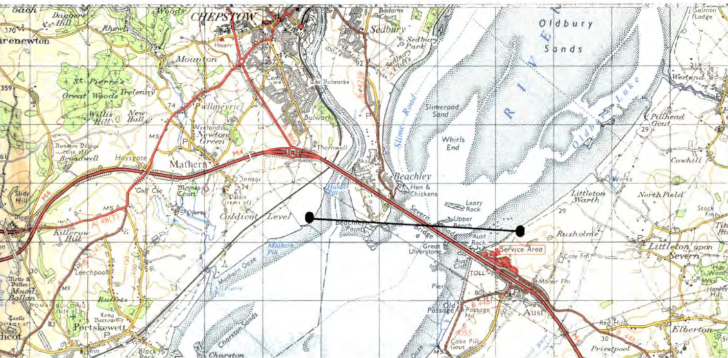
Map 33. Route of proposed 400 kV cable tunnel under the River Severn between Aust and Caldicot Level.
