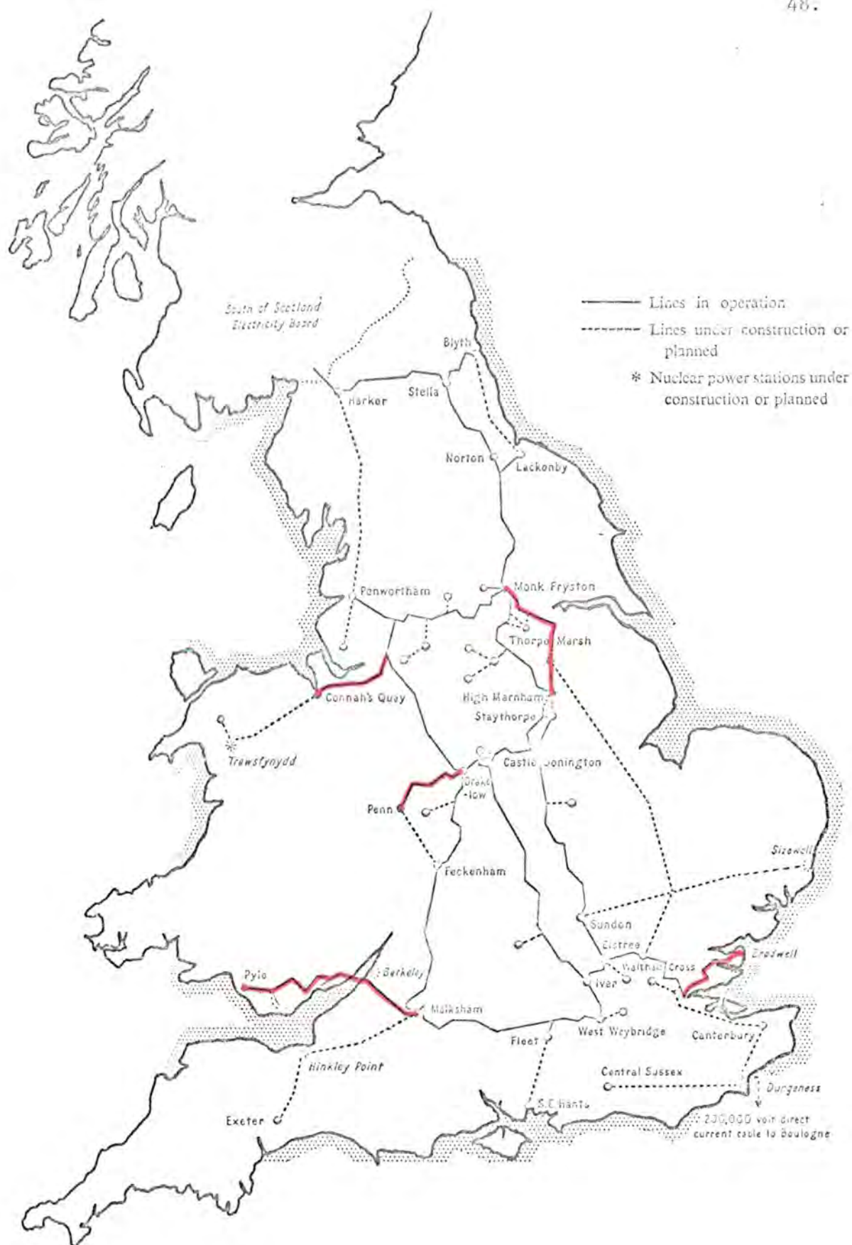
Map No. 4 - 275 kV Supergrid in 1960. Lines in red indicate the additional circuits to those proposed in 1951.
