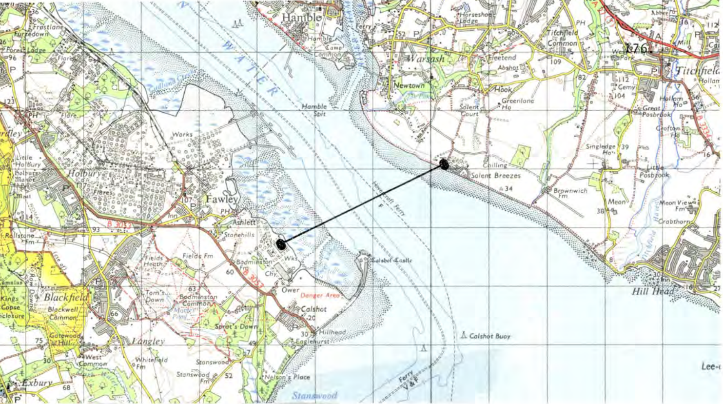
Map 29. Route of 400 kV cable tunnel under Southampton Water between Fawley Generating Station and Chilling.
