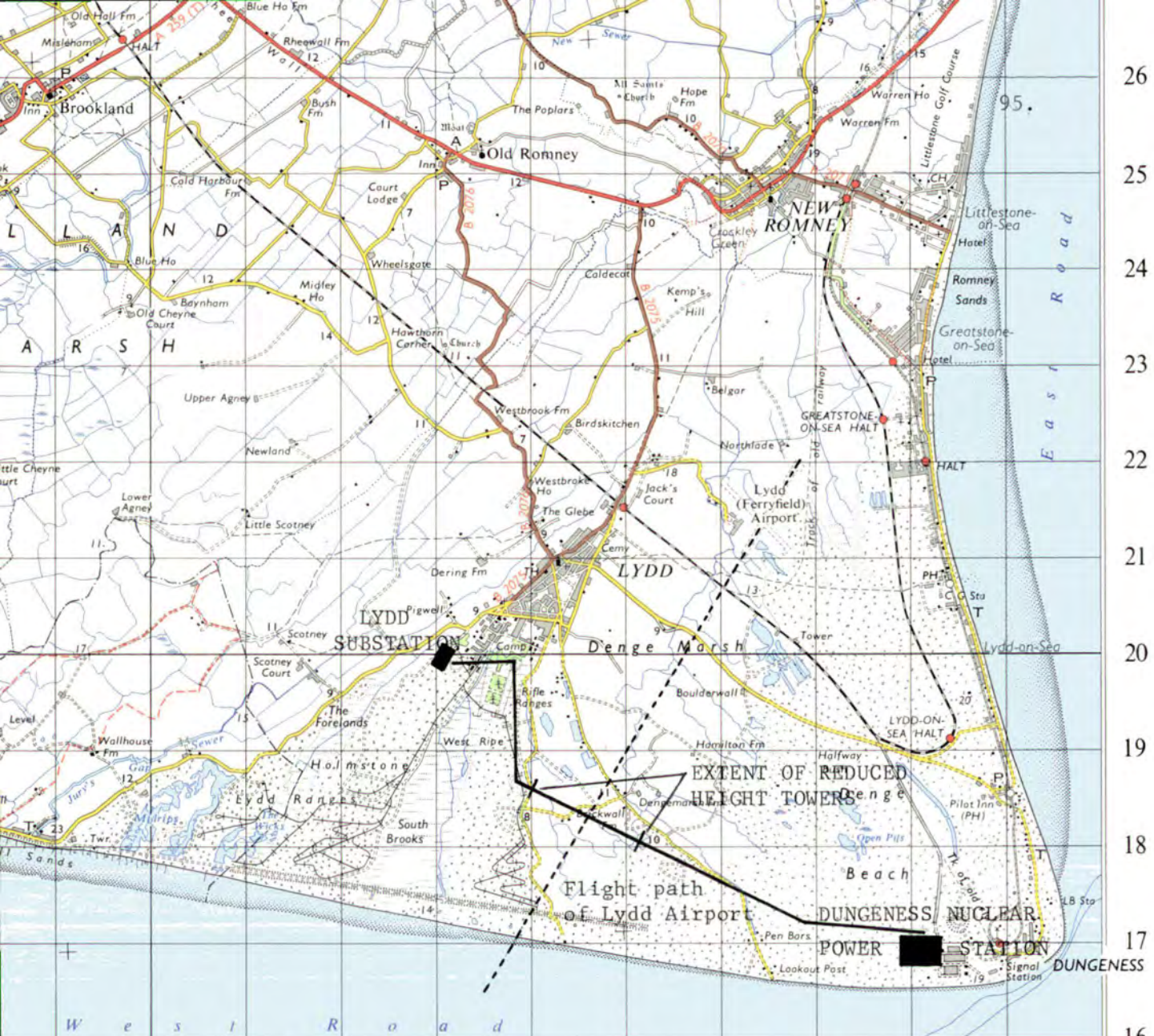
MAP 15 REDUCED HEIGHT TOWERS TO PROVIDE SAFETY CLEARANCE FOR AIRCRAFT APPROACHING OR LEAVING THE MAIN RUNWAY OF LYDD AIRPORT
