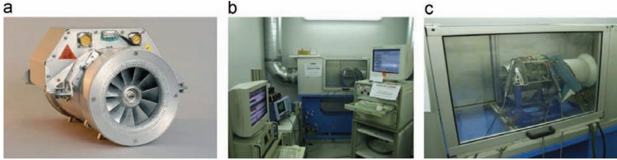
Fig. 1. (a) TECHNOfan LP2 fan, (b) and (c) bearing fault diagnostic experimental test bench.
