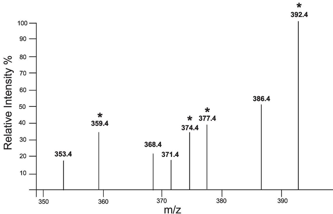
FIGURE 3. Averaged mass-spectral DI/EI-SIM data (50 scans) for a standard mixture of cholesterol and  $D_6$ -cholesterol (1:2, wt/wt). Ions at  $m/z$  386.4, 371.4, 368.4, and 353.4 represent the  $M^+$ ,  $[M-15]^+$ ,  $[M-18]^+$ , and  $[M-33]^+$  diagnostic ions for cholesterol, respectively. Ions at  $m/z$  392.4, 377.4, 374.4, and 359.4 (asterisk) correspond to the deuterated analogues arising from  $D_6$ -cholesterol.
