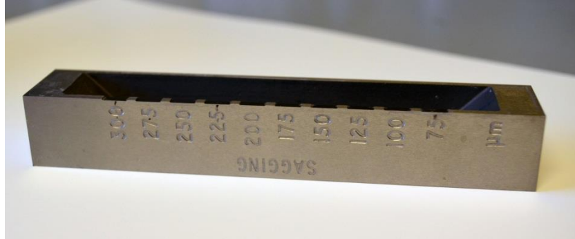
Figure II.3. Multifilm thickness bar used to drawdown the wet films on Lenetta panels.
