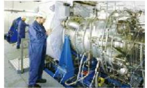
SGT-400 core engine test facility.
