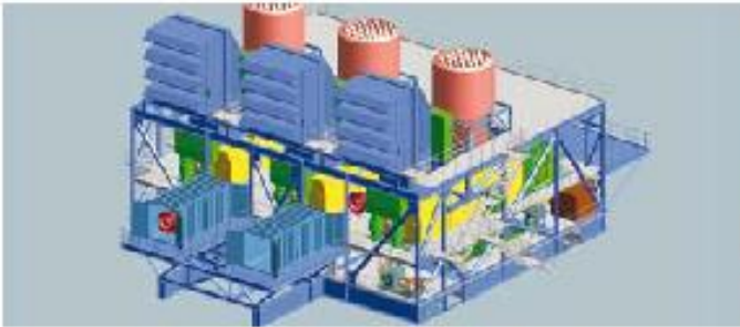
Standard single-lift power generation module for floating platforms.
