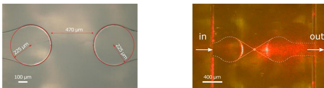
Fig. 5.3: (Left) Discontinuous waveguide with curved end-faces with a radius of curvature of 225 \mu\text{m} ; (right) propagation of light with a wavelength of 650 \text{ nm} through a light-fluid interaction region in a microcuvette. The microscopic pictures are obtained using a digital microscope Keyence VHX-5000.
