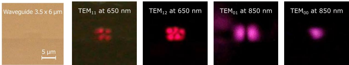
Fig. 4.13: Digital microscope pictures of the 3.5 \times 6 \mu\text{m}^2 waveguide operating in few mode regime. From left to right: polished waveguide core end-face without light, TEM_{11} and TEM_{12} at the wavelength of 650 nm; TEM_{00} and TEM_{01} at \lambda = 850 nm.
