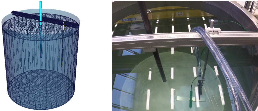
Figure 6.1: Left: Wire mesh model of the CARROUSEL facility. Right: Picture from above on the CARROUSEL tank with internals of the experiment visible.
