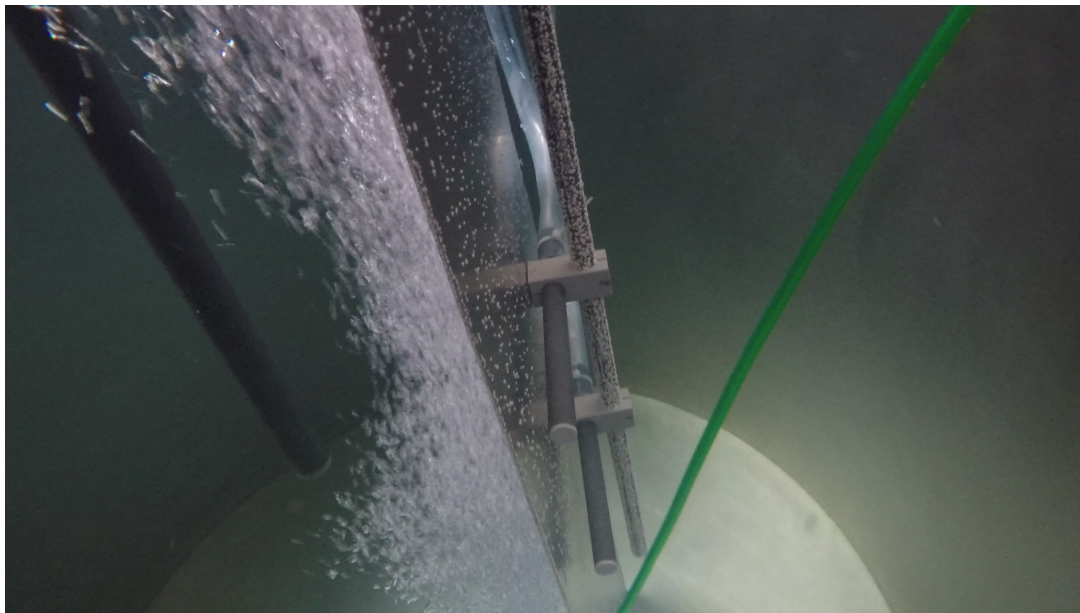
Figure 6.8: Picture of the experimental setup III at 10 lpm with added aluminium plate with the aim to reduce vibrations induced by the bubbles.
