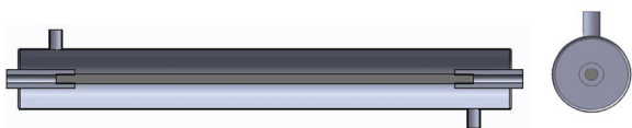
Figure 1. One lamp cylindrical reactor with negative irradiation geometry, longitudinal and transverse cross section.
