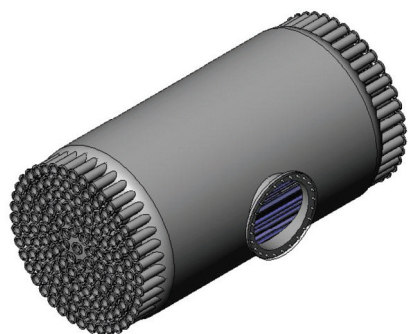
Figure 4. High capacity cylindrical multilamp reactor with negative irradiation geometry (above 1 m 3 /s).
