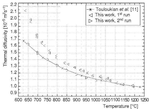
**Figure 4. Thermal diffusivity of uncoated silicon specimen (1<sup>st</sup> run) and silicon specimen coated with a metallic layer (2<sup>nd</sup> run)**
