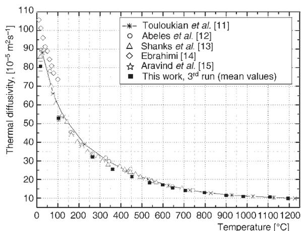
**Figure 5. Thermal diffusivity of silicon specimen coated with colloidal graphite (3<sup>rd</sup> run)**
