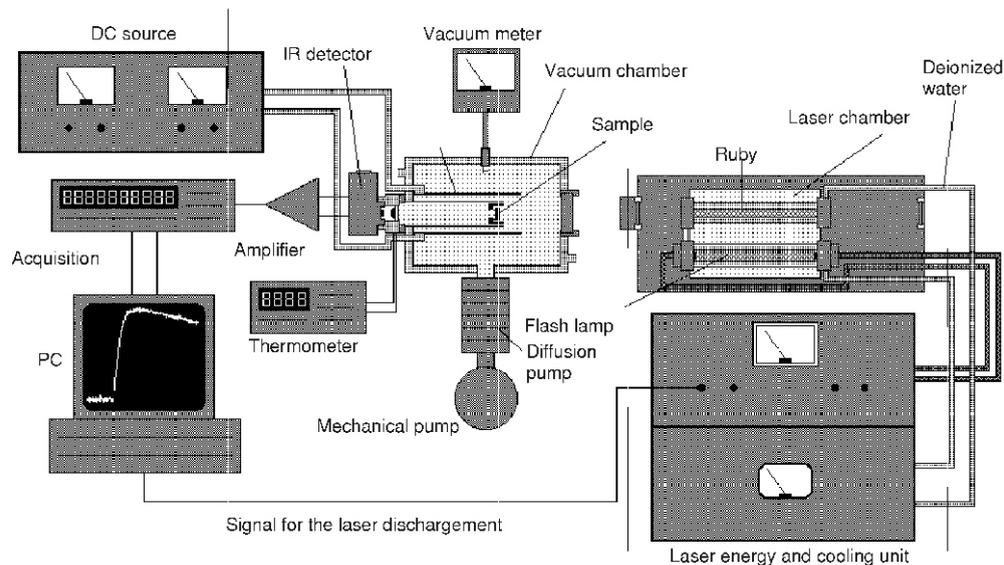
Figure 1. Schematic diagram of applied laser flash apparatus
