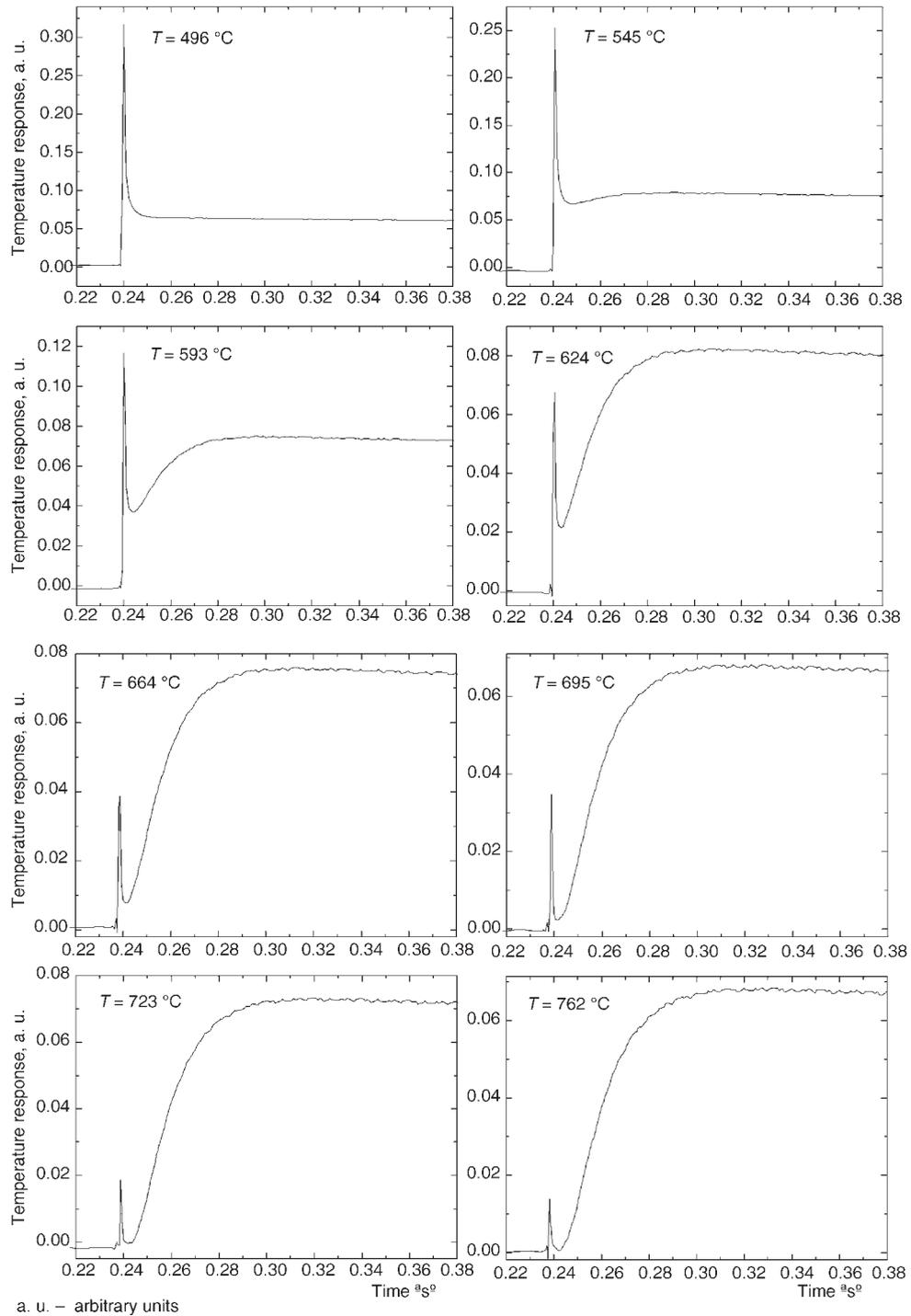
**Figure 3. Temperature responses of uncoated silicon specimen**
