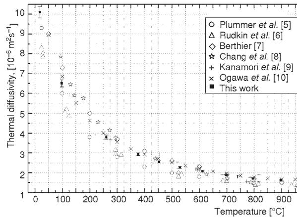
**Figure 2. Thermal diffusivity of coated alumina specimen**
