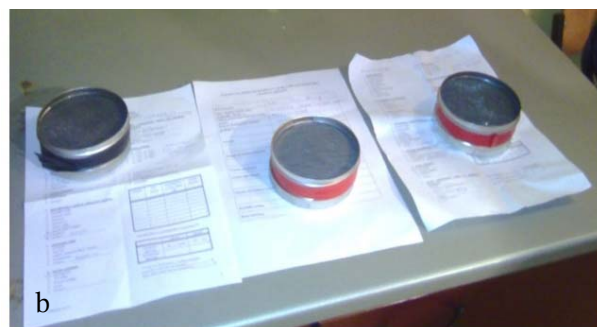
Fig. 1. (a) Charcoal canister assembly [3] and (b) photo of canisters' exposure during interlaboratory comparison in 2015.
