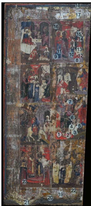
Slika 2. Mesta EDXRF merenja na levoj polovini ikone. Figure 2. Positions on the left half of the icon where EXDRF measurements were performed.
