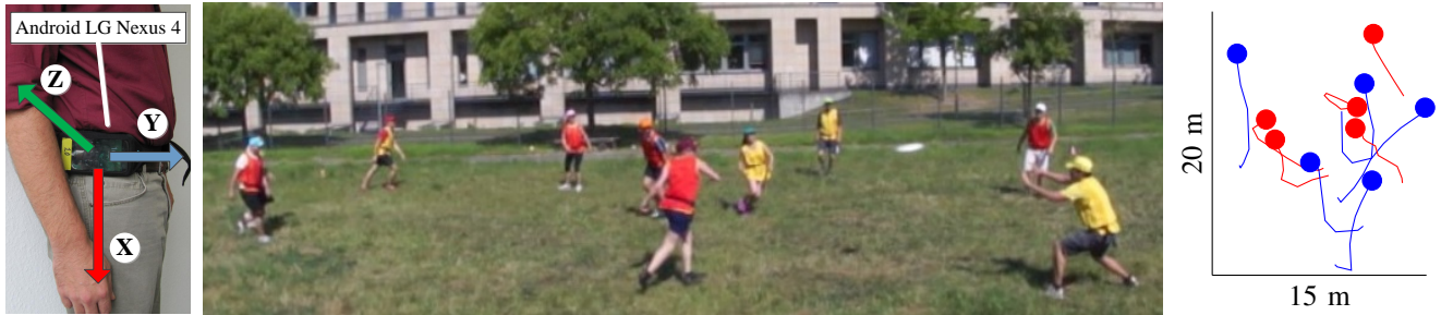
Fig. 3. Device Placement (Left) for the Team Sports Group Activity Experiment (Middle) with Relative Subject Locations on the Field (Right)
