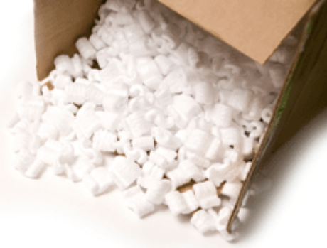
Figure 21: ReBioFoam: biodegradable biopolymer foam and biobased to be used as a solution for protective packaging in alternative to foamed materials of synthetic origin [Greenews, 2013]
