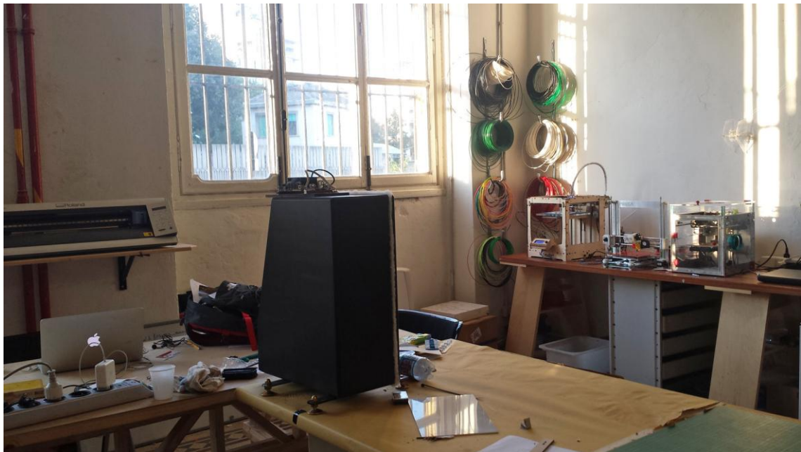
Figure 26: A view from the FabLab Torino premises, showing their two 3D printers (the two boxes on the right) and the cutting plotter (on the very left).
