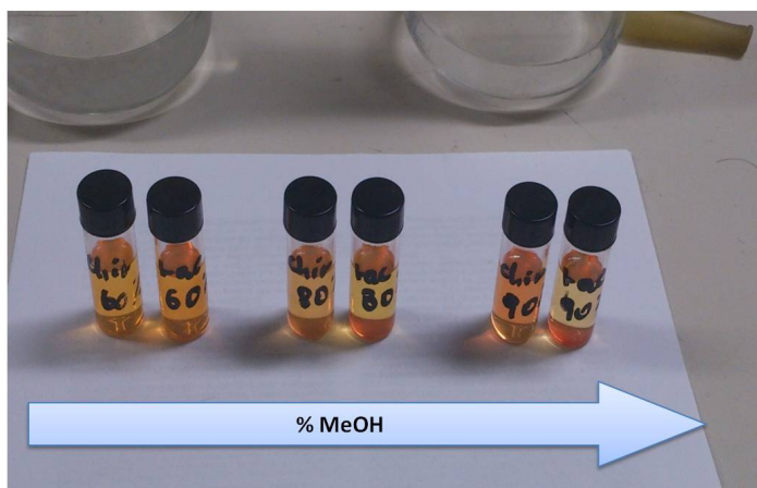
FIGURE 20: SAMPLES OF LOW MOLECULAR WEIGHT ( R )-MEH-PPV (ON THE LEFT OF EACH PAIRS) AND MEH-PPV (ON THE RIGHT) WITH INCREASING AMOUNTS OF NON-SOLVENT, 18 HOURS THEIR PREPARATION
