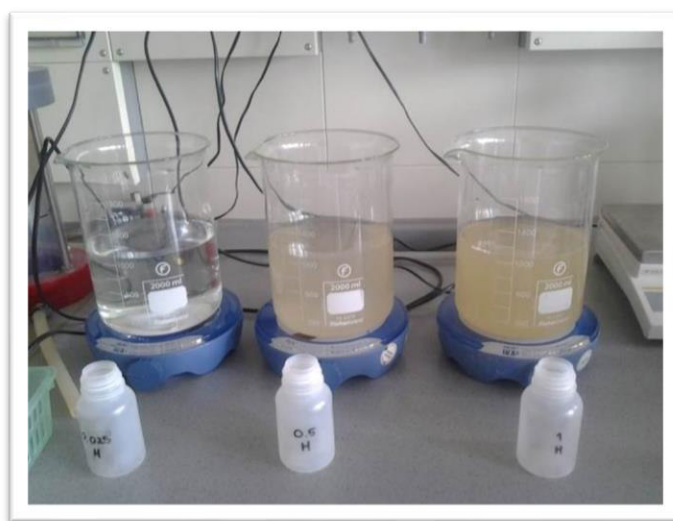
Figure 16. Artificial raw water created from a mixture of natural soil and tap water under varied concentration. The most transparent water has the lowest concentration of suspended solids and turbidity value.
