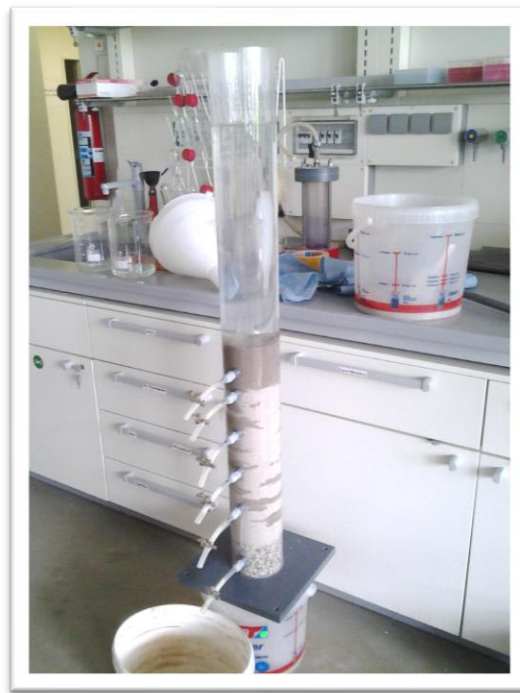
Figure 15. Short circuiting in the filter column
