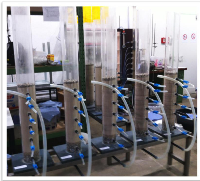
Figure 21. Phase I - Construction of filter columns in Set 1
