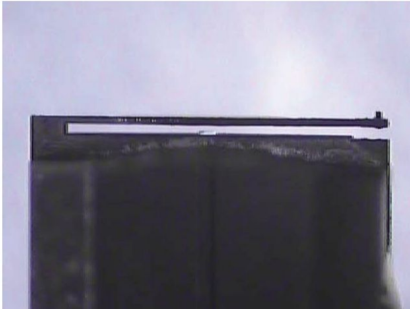
Figure 5.4: Optical microscope image of a tipped ferrule-top cantilever.
