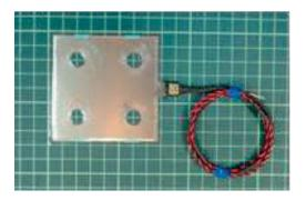
Fig. 3.8 60×60mm prototype pad sensor
