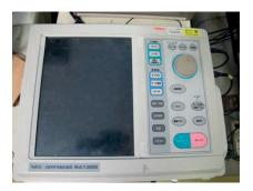
Fig. 3.11 High-speed voltage recorder
