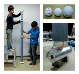
Fig. 4.4 Ball falling test on the column sensor
