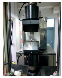
Fig. 3.10 200kN servo-hydraulic testing machine
