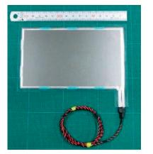
**Fig. 4.1** Example of pad sensor
