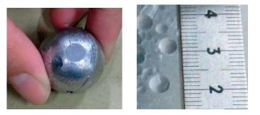
Fig. 3.18 Deformation on the ball and surface of sensor
