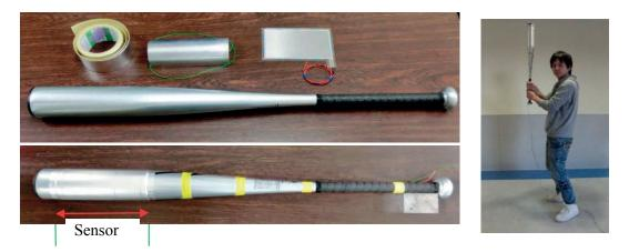
Fig.4.7 Baseball bat before and after the setting of pipe sensor
