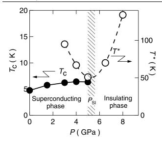
FIG. 3. The superconducting transition temperature  $T_{\rm c}$  and the characteristic temperature  $T^*$  plotted as functions of pressure. The solid and broken lines are guides to the eyes. Superconductivity vanishes at  $P_{\rm SI}$ , where  $T^*$  has the minimum value and the metal-insulator phase boundary (hatched) is expected to lie.
