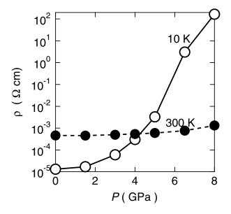
FIG. 2. Pressure dependence of electric resistivity  $\rho(T)$ . The open and closed circles represent  $\rho(10 \text{ K})$  and  $\rho(300 \text{ K})$ , respectively. Each point was taken from the experimental data shown in Fig. 1(a). Both  $\rho(10 \text{ K})$  and  $\rho(300 \text{ K})$  basically increase monotonically with pressure, although an inflection point is seen in  $\rho(10 \text{ K})$  between 5.0 and 6.5 GPa.
