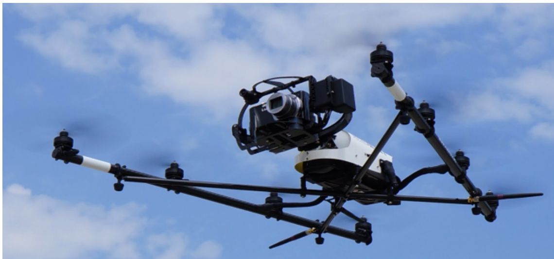
Figure 3. UAV AscTec Falcon 8 model with mounted Panasonic DMC Lumix LX3 cameras
