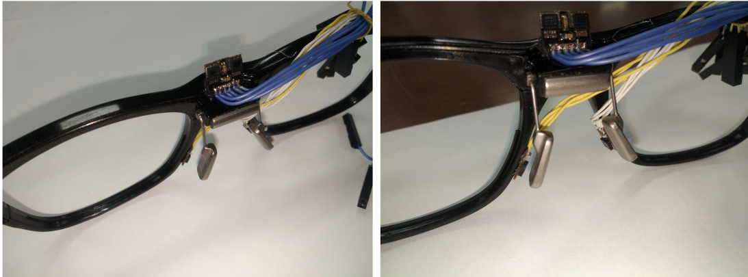
Figure 7.1: J!NS Meme with additional infrared sensors for measuring facial temperature in the forehead and nose-tip region.
