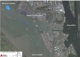
Figure 1 : Port Of Antwerp ; Location North Sea Terminal; Three examples of passing trajectories (blue) and edge of navigational channel (green dash). – image courtesy of Antwerp Port Authority
