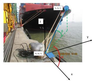
Figure 3 : Definition line angles  $\alpha$  and  $\beta$  and the length of the line section between bollard and fairlead (*l*).
