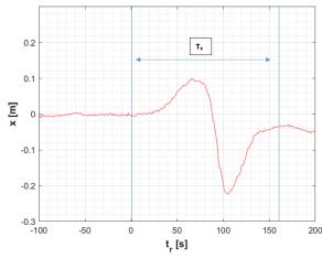
Figure 2 : GPS registration longitudinal motion of moored Neo-Panamax container vessel with passing oil tanker.
