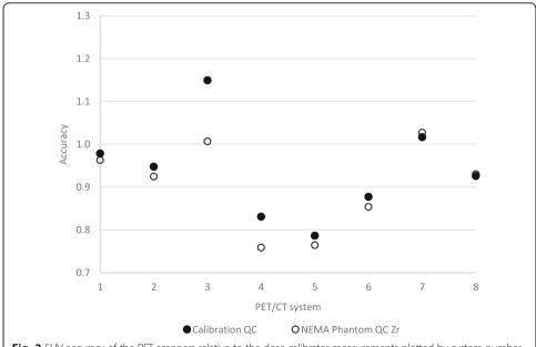
**Fig. 2** SUV accuracy of the PET scanners relative to the dose calibrator measurements plotted by system number. Systems 1–2 and 3–4 represent GE scanners Discovery 690 and Discovery 710, respectively; systems 5–6 are Siemens Biograph 40\_mCT and Somatom Definition AS\_mCT; system 7 is the Phillips Ingenuity TF PET/CT; system 8 is the Siemens Biograph 64\_mCT
