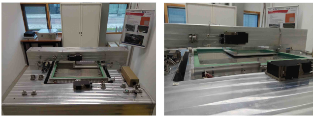
Figure 1: The moving-magnet prototype (NAPAS)
