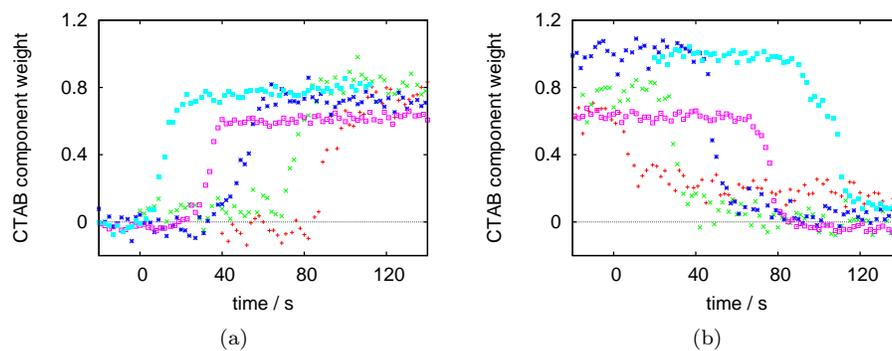
Figure S.1: CTAB kinetics for 0.47 mM (red +), 0.75 mM (green ×), 1.0 mM (blue \*), 4 mM (pink □), 10 mM (turquoise ■). (a) Adsorption kinetics, (b) desorption kinetics. The curves have been offset on the time axis for ease of viewing. The kinetics are presented in terms of component weight (normalised to water) rather than surface excess owing to the uncertainty in the calibration factor.
