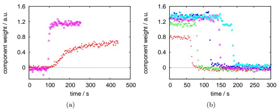
Figure S.2: (a) Adsorption and (b) desorption kinetics of TX-100 onto cellulose. Concentrations are 0.2 mM (red +), 0.4 mM (green ×), 1.0 mM (blue \*), 4 mM (pink ◻) and 10 mM (turquoise ◼). The different runs have been offset on the time axis for ease of viewing. The kinetics are presented in terms of component weight (normalised to water) rather than surface excess owing to the uncertainty in the calibration factor.
