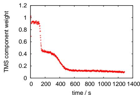
Figure 6: Kinetics of removal of TMS from cellulose. Sy polarisation, 1 s acquisition time per point, flow rate of HCl solution =  $0.5 \text{ mL min}^{-1}$ . Only the TMS component is plotted; the cellulose/water component varied by less than 20% over the course of the experiment.
