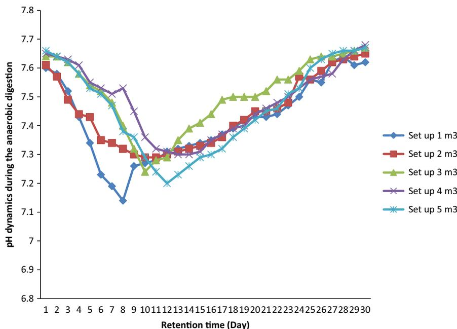
**Fig. 1.** Graph of pH dynamics during the anaerobic digestion (for the first five experimental set ups).
