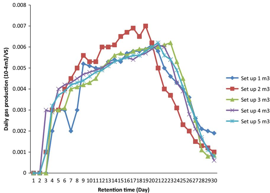
Fig. 2. Daily biogas production during the anaerobic digestion (from the first five experimental set ups).
