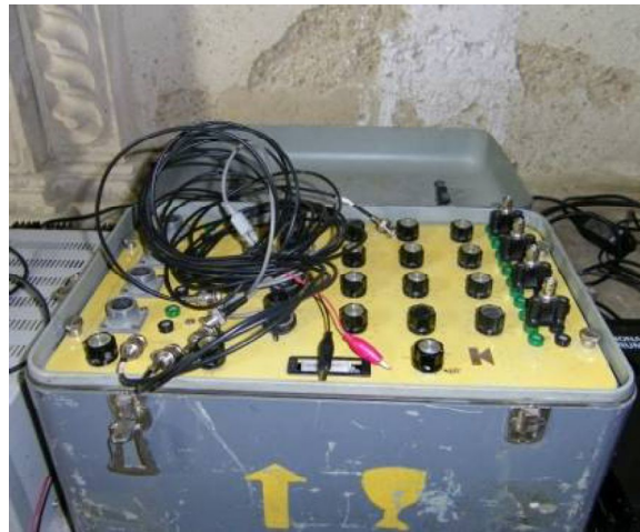
Figure 12 Equipment for ambient vibration measurements: the four channel signal conditioner (see online version for colours)
