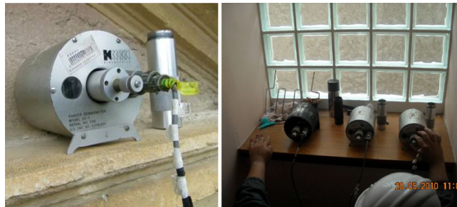
Figure 12 Equipment for ambient vibration measurements: the four channel signal conditioner (see online version for colours)
