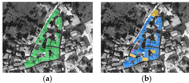
Figure 12. Damage maps: (a) E.D. = 20 km and M = 4 and 5; (b) E.D. = 20 km and M = 6.
