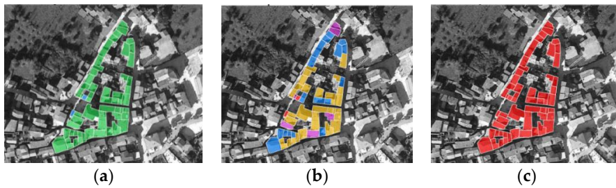
Figure 10. Damage maps: (a) E.D. = 5 km and M = 4; (b) E.D. = 5 km and M = 5; (c) E.D. = 5 km and M = 6.
