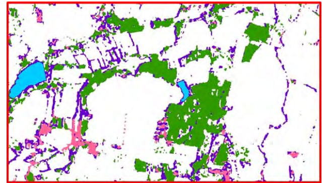
figure 5: TerraSar X unsupervised classification (green woods and riparian, purple: hedgerows, pink: built area/ mineral surface, blue: water)
