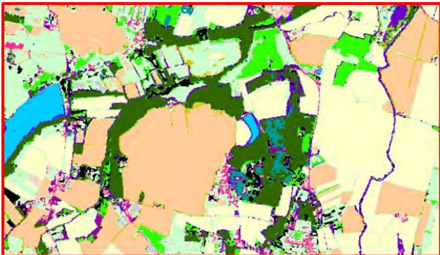
figure 3: Formosat-2 unsupervised classification (green: woods and riparian, purple: hedgerows, pink: built area/ mineral surface, light green: grassland, yellow and orange: winter and summer crop, blue: water)
