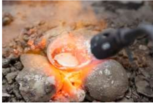
Figure 309 Melting process of the silver © Khalid Al Busaidi
