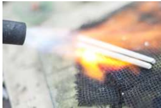
Figure 310 Annealing of the steel strips © Khalid Al Busaidi
