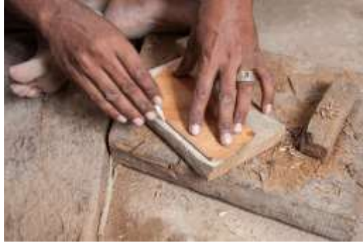
Figure 216 Marking the shape of the scabbard core © Khalid Al Busaidi
