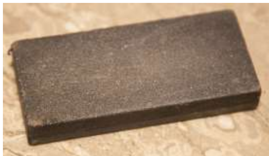
Figure 354 A silicon carbide abrasive block with different grits on upper and lower faces © Khalid Al Busaidi
