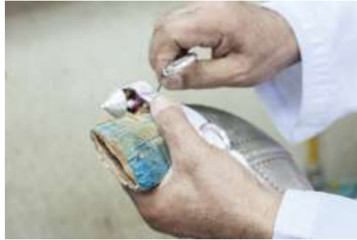
Figure 303 Inserting the rivets by attaching the rings © Khalid Al Busaidi
