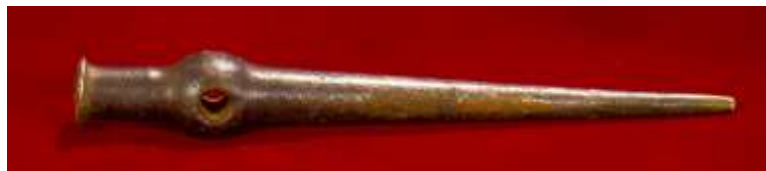
Figure 415 Ring stick used for making rings for belt holder and belt © Khalid Al Busaidi
