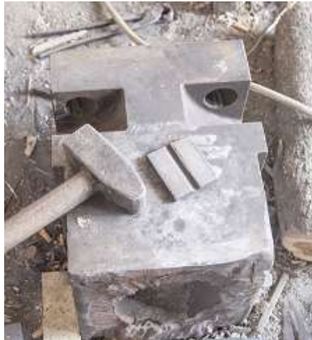
Figure 364 Steel section used as an anvil © Khalid Al Busaidi
