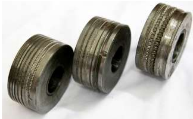
Figure 395 Examples of embossing rollers for creating decoratively patterned wire © Khalid Al Busaidi
