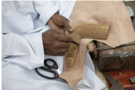
Figure 235 Marking the shape of a scabbard core using an additional material © Khalid Al Busaidi
