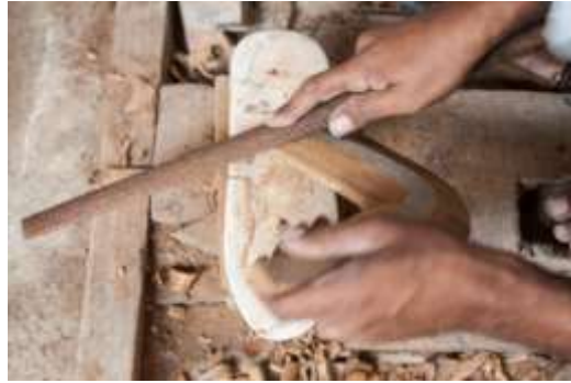
Figure 228 Smoothing of a scabbard core using a rasp © Khalid Al Busaidi
