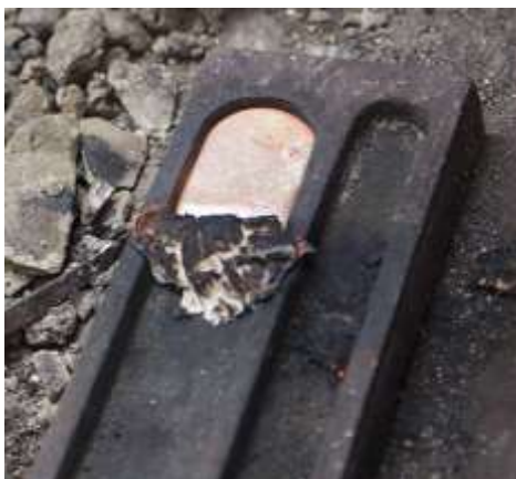
Figure 385 Mould for creating small billets of silver or gold © Khalid Al Busaidi
