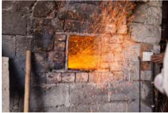
Figure 191 Air is supplied by a fan after heating the furnace using diesel © Khalid Al Busaidi
