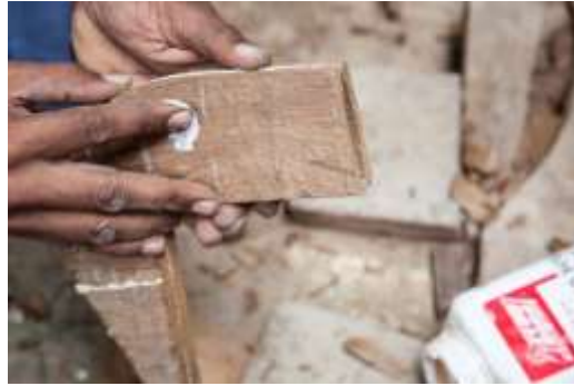
Figure 225 Glueing of the scabbard core together © Khalid Al Busaidi
