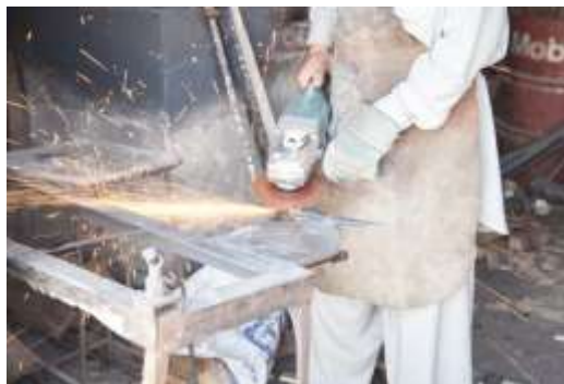
Figure 205 Cutting of the blade to an appropriate shape and trimming the spine and tang © Khalid Al Busaidi
