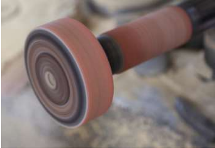
Figure 371 Small electrically powered rotary sanding machine © Khalid Al Busaidi
