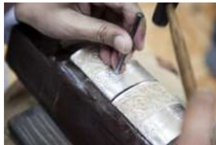
Figure 263 Embossing and engraving using small steel tools © Khalid Al Busaidi
