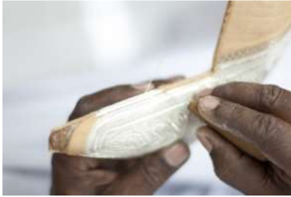
Figure 245 Sewing the front and back of the scabbard covers with silver wire © Khalid Al Busaidi
