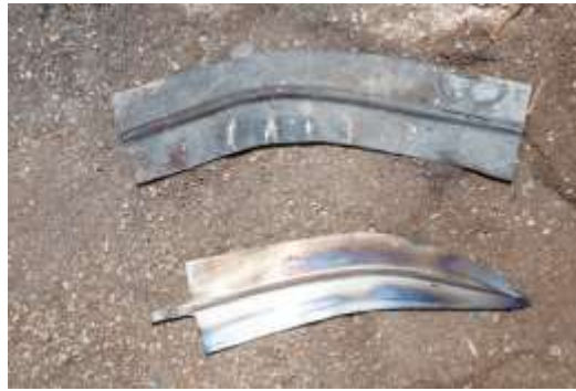
Figure 207 Forged and curved blade section before and after trimming to a particular shape. © Khalid Al Busaidi
