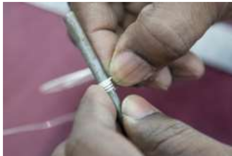
Figure 266 Winding silver wire around tube to form spiral rings © Khalid Al Busaidi
