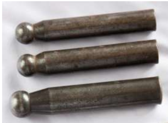
Figure 396 Round-headed and hardened steel swages © Khalid Al Busaidi
