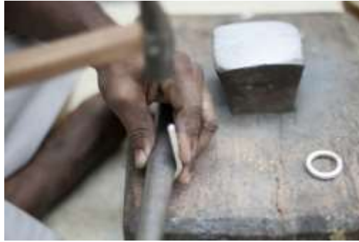
Figure 312 Wrapping of silver around a steel former © Khalid Al Busaidi
