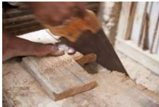
Figure 217 Removing the excess wood with a handsaw © Khalid Al Busaidi
