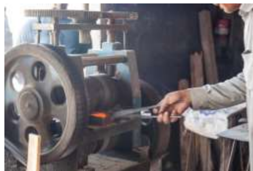
Figure 199 A partly roll forged blade after reheating © Khalid Al Busaidi
