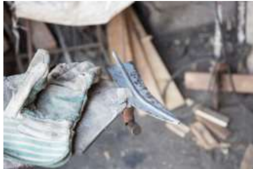
Figure 208 Clamp for holding khanjar blades for cutting and grinding © Khalid Al Busaidi
