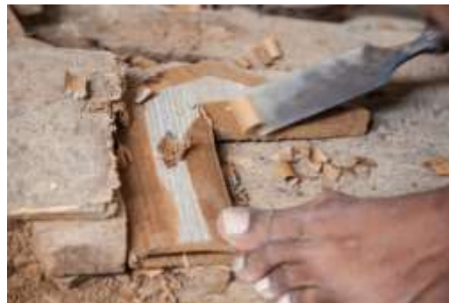
Figure 226 Trimming of a scabbard core with a chisel © Khalid Al Busaidi
