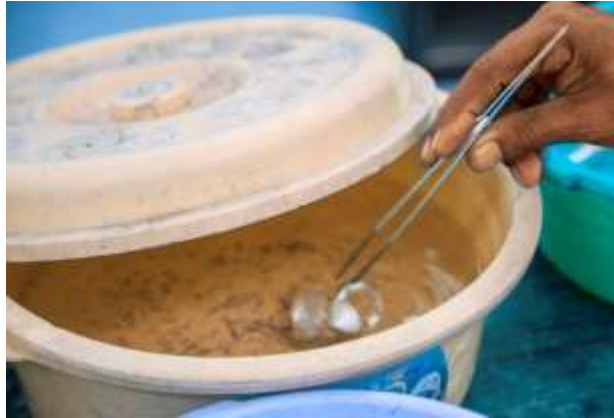
Figure 452 Using battery acid to clean khanjar parts © Khalid Al Busaidi
