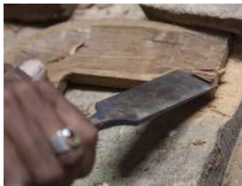
Figure 374 Chisel being used to cut central cavity of side of the khanjar scabbard core © Khalid Al Busaidi
