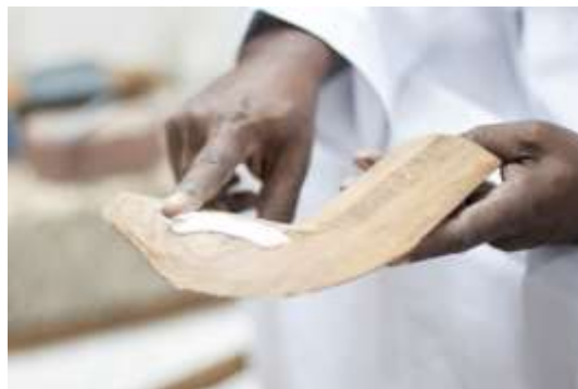
Figure 242 Starting glueing the scabbard cover to the scabbard core © Khalid Al Busaidi
