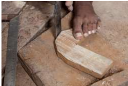
Figure 218 Chopping the rough cut towards the final outline using a chisel © Khalid Al Busaidi
