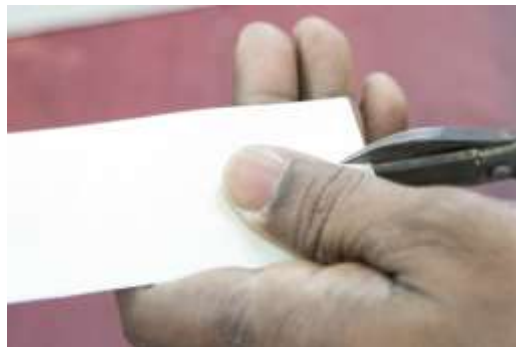
Figure 253 Cutting of the silver sheet © Khalid Al Busaidi
