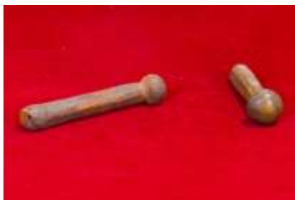
Figure 277 Small steel hardies used for hammering the chape to shape © Khalid Al Busaidi
