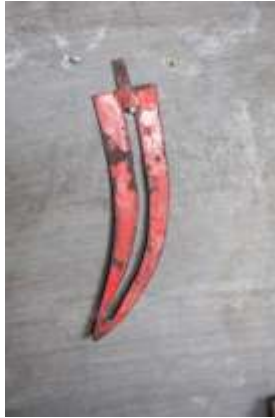
Figure 204 Blade shaper with an appropriate size pattern © Khalid Al Busaidi
