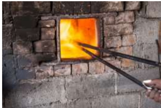
Figure 192 Inserting the steel piece that will become the khanjar blade © Khalid Al Busaidi
