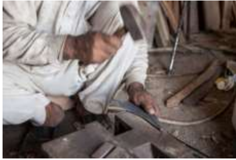
Figure 210 Straightening the inner curve of the blade © Khalid Al Busaidi
