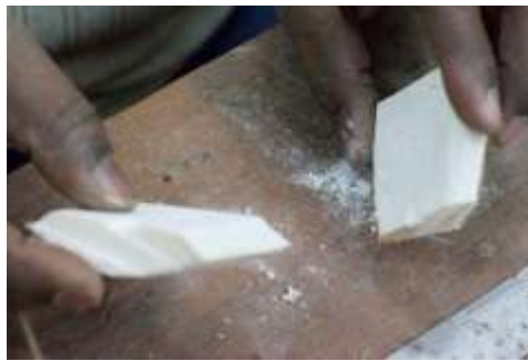
Figure 335 Cuttlefish bone cut into two matching parts © Khalid Al Busaidi
