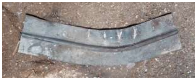
Figure 203 Blade section after bending with a hand forging tool © Khalid Al Busaidi
