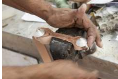
Figure 297 Clamping the glued belt holder © Khalid Al Busaidi
