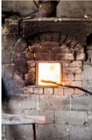
Figure 193 Steel piece of khanjar blade being removed after heating © Khalid Al Busaidi
