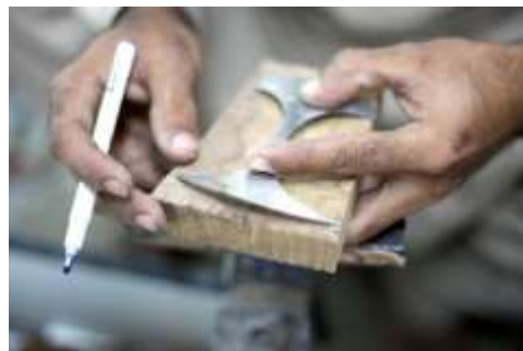
Figure 166 Comparing wood pieces to a template for the silver handle face © Khalid Al Busaidi
