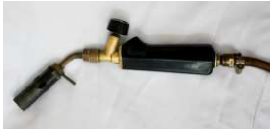
Figure 429 Gas torch © Khalid Al Busaidi
