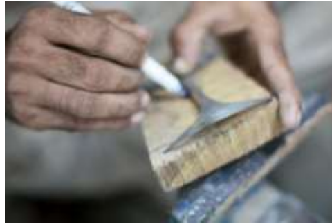
Figure 167 Marking the silver faceplate area and the handle outline © Khalid Al Busaidi
