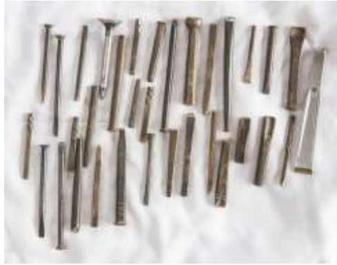
Figure 393 Embossing and engraving tools © Khalid Al Busaidi
