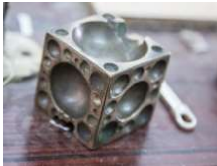
Figure 316 Tool used in making conical shaped rings © Khalid Al Busaidi
