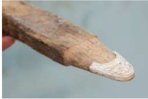
Figure 278 Hardwood standard former for chape shown fitted with a fully completed chape © Khalid Al Busaidi
