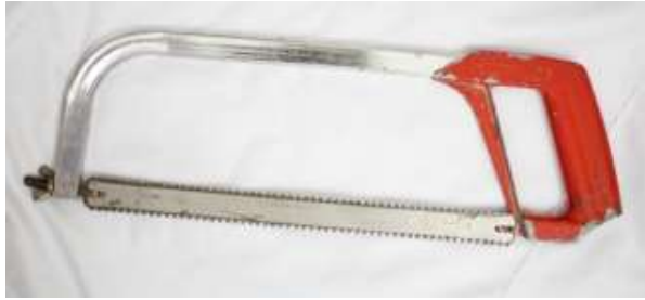
Figure 373 Adjustable tension handsaw with coarse tooth blade © Khalid Al Busaidi
