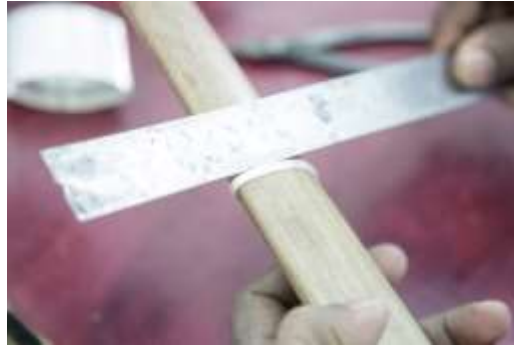
Figure 259 Adjusting the size and shape of a silver ring using a hardwood former © Khalid Al Busaidi
