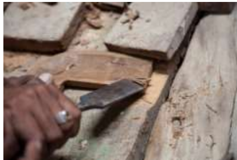
Figure 223 Carving of the blade cavity in one of the sides of the scabbard core © Khalid Al Busaidi
