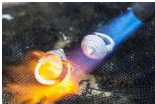
Figure 317 Soldering the conical heads to the rings © Khalid Al Busaidi
