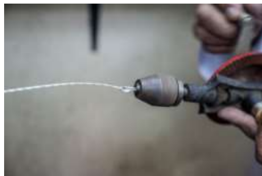
Figure 322 Starting twisting the wire © Khalid Al Busaidi
