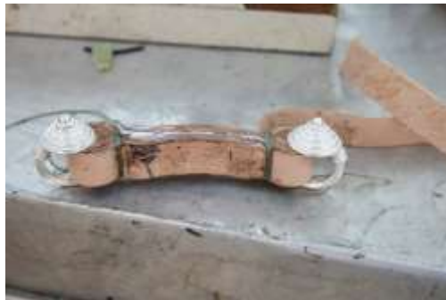
Figure 298 Lashing the ends of the belt holder © Khalid Al Busaidi
