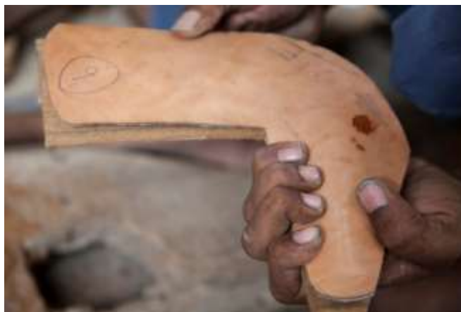
Figure 229 Checking the size and shape of a scabbard core © Khalid Al Busaidi
