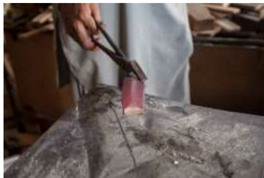
Figure 194 Steel piece just after removal from the furnace © Khalid Al Busaidi
