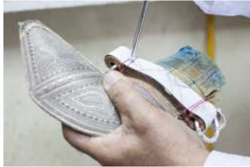
Figure 300 Making holes for attaching the belt holder © Khalid Al Busaidi
