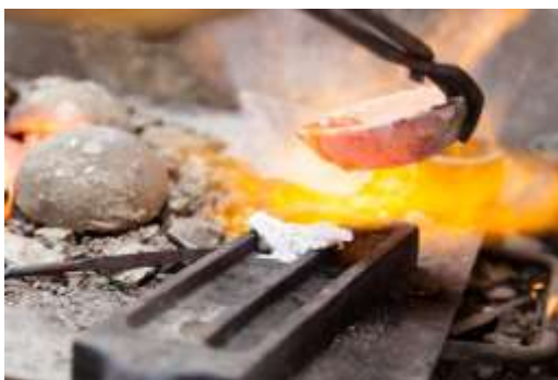
Figure 249 Pouring silver into the standard mould to make a billet © Khalid Al Busaidi
