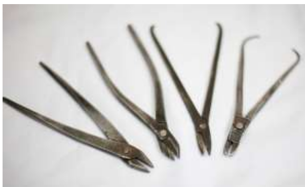
Figure 389 Pliers, shears, snips and pincers © Khalid Al Busaidi
