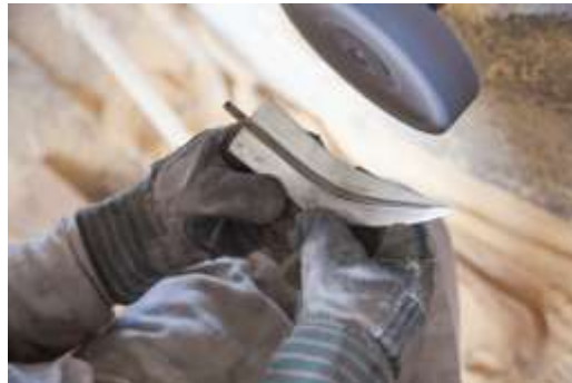
Figure 214 Khanjar blade in the process of being smoothed and polished all over © Khalid Al Busaidi
