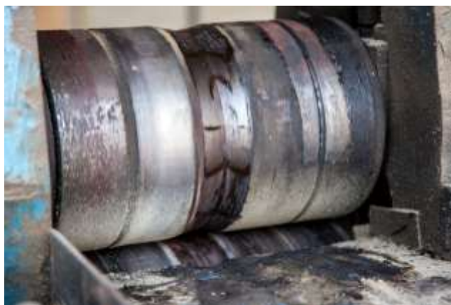
Figure 361 Upper roll of electrically powered small roll forging machine © Khalid Al Busaidi
