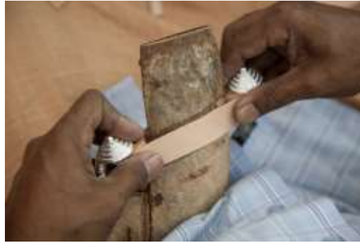
Figure 294 Measuring the length of the loop around the scabbard and the rings © Khalid Al Busaidi
