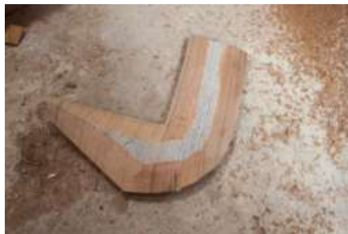
Figure 227 A scabbard core in final rough form © Khalid Al Busaidi
