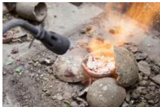
Figure 248 Melting process of silver © Khalid Al Busaidi
