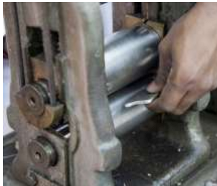
Figure 387 Piece of silver being fed into pressure rolling machine © Khalid Al Busaidi
