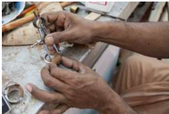
Figure 284 Using dividers to measure the maximum width of the belt holder © Khalid Al Busaidi
