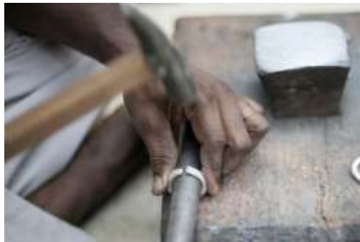
Figure 313 Hammering process of the ring to a particular shape © Khalid Al Busaidi
