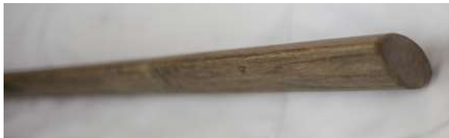
Figure 391 Wooden former for sizing and shaping the ferrule and scabbard upper cover © Khalid Al Busaidi
