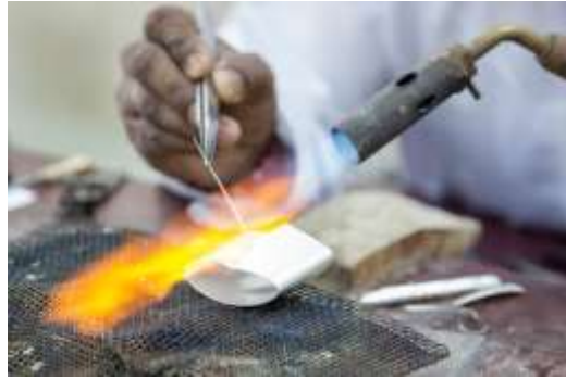
Figure 257 Silver soldering process of the edges of the back of the upper scabbard cover © Khalid Al Busaidi
