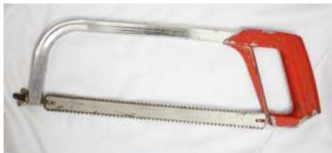
Figure 348 Adjustable tension handsaw with coarse tooth blade © Khalid Al Busaidi
