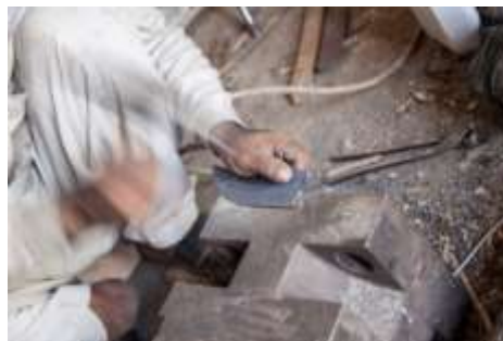
Figure 209 Straightening the outside of the blade © Khalid Al Busaidi
