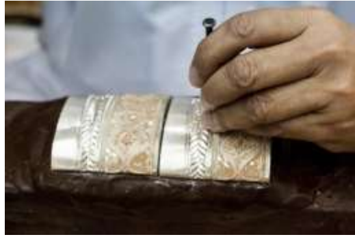
Figure 450 Khanjar pieces held in resin while being embossed and engraved © Khalid Al Busaidi
