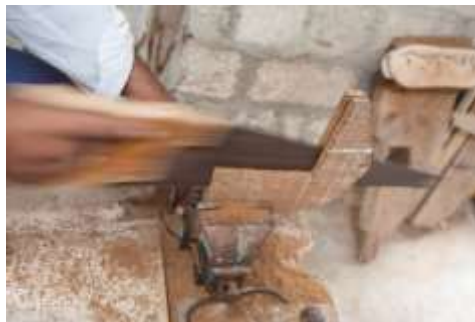
Figure 221 Cutting the scabbard into two pieces using a handsaw © Khalid Al Busaidi
