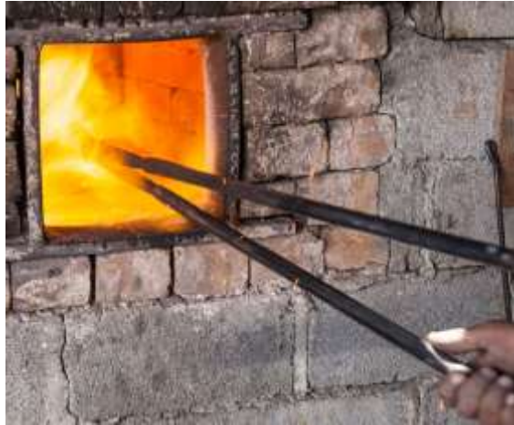
Figure 360 Tongs inserting steel piece into drip oil furnace with fan forced air supply off © Khalid Al Busaidi
