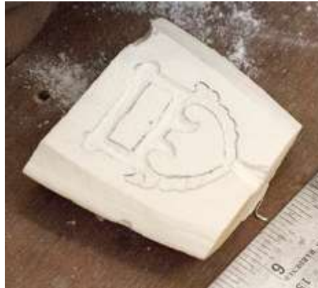
Figure 420 A cuttlefish bone mould for a belt buckles © Khalid Al Busaidi
