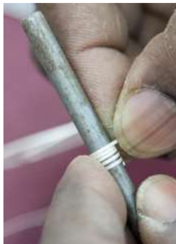
Figure 398 Steel tubing used for wrapping silver or gold wire into spirals for Al Takisir © Khalid Al Busaidi
