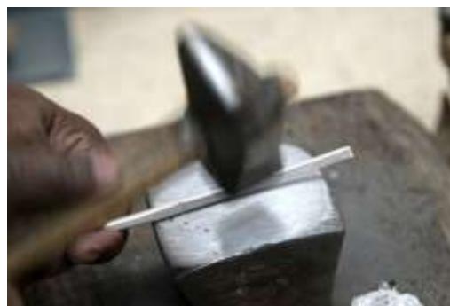
Figure 311 Forming of the strips for rings © Khalid Al Busaidi
