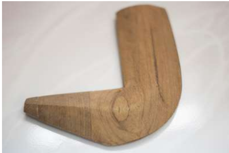
Figure 130 Carved hollow wooden scabbard core after gluing and ready to have other elements attached © Khalid Al Busaidi
