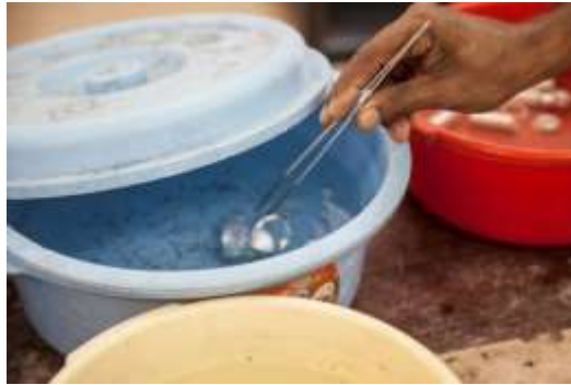
Figure 318 Placing of newly soldered rings in water © Khalid Al Busaidi
