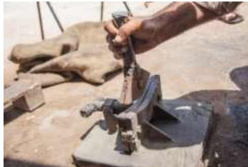
Figure 202 Curve handed blade forging tools © Khalid Al Busaidi
