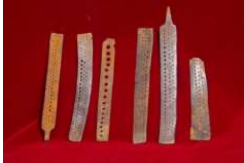
Figure 326 Handmade drawing dies for reducing the thicknesses of wire © Khalid Al Busaidi
