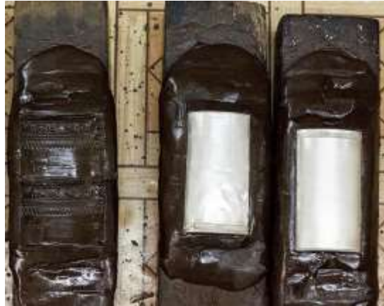
Figure 392 Wooden holder for embossing and engraving silver and gold sheet items © Khalid Al Busaidi
