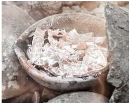
Figure 382 Crucible with small pieces of silver being heated © Khalid Al Busaidi
