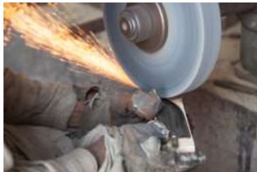
Figure 211 Using fine grinding wheel on khanjar blade for initial sharpening © Khalid Al Busaidi
