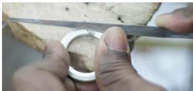
Figure 413 Triangular file being used to smooth soldered joint on silver ring © Khalid Al Busaidi
