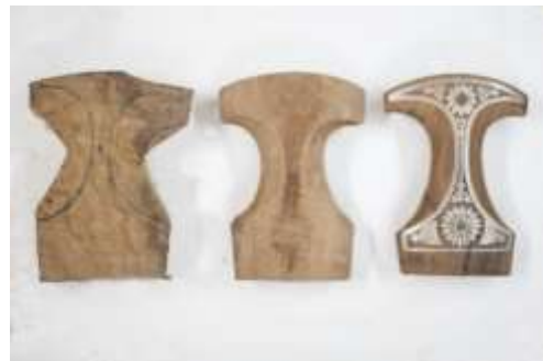
Figure 172 Sequence of creating a handle from rough cut to decoration © Khalid Al Busaidi
