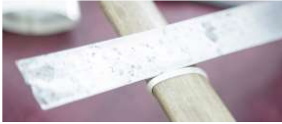
Figure 388 Using a ruler to tap a silver ring along a tapered former to increase its size © Khalid Al Busaidi
