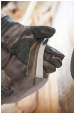
Figure 213 Inner curve of blade smoothed and polished using grinding wheel © Khalid Al Busaidi
