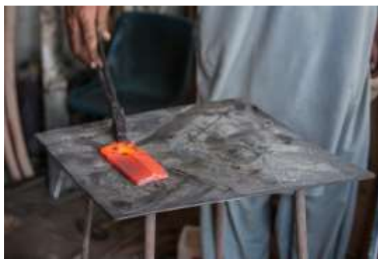
Figure 198 A partly forged blade after reheating © Khalid Al Busaidi
