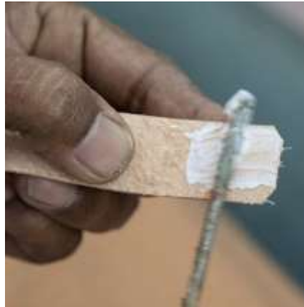
Figure 404 Steel tube used to spread glue © Khalid Al Busaidi
