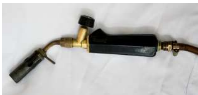
Figure 408 Gas torch © Khalid Al Busaidi
