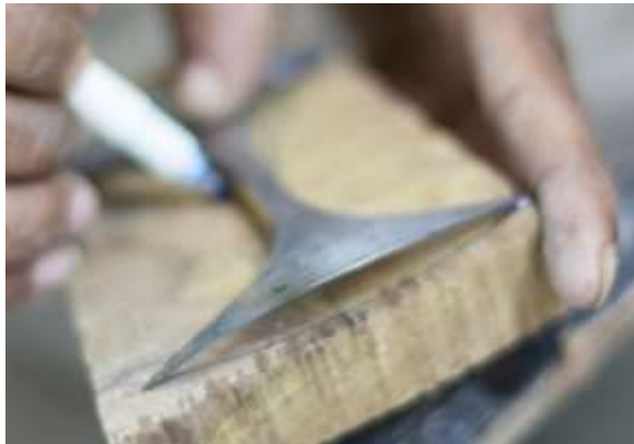
Figure 345 Use of a pen to mark out the shape of a khanjar handle © Khalid Al Busaidi
