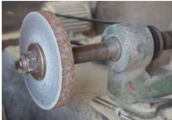
Figure 370 An electric bench-mounted grinding wheel © Khalid Al Busaidi
