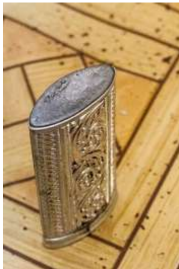
Figure 447 Lead filling scabbard upper cover for embossing © Khalid Al Busaidi
