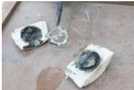
Figure 339 Removing the buckle from the mould © Khalid Al Busaidi
