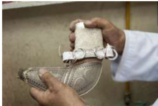
Figure 274 Checking the fitness of the scabbard upper cover © Khalid Al Busaidi
