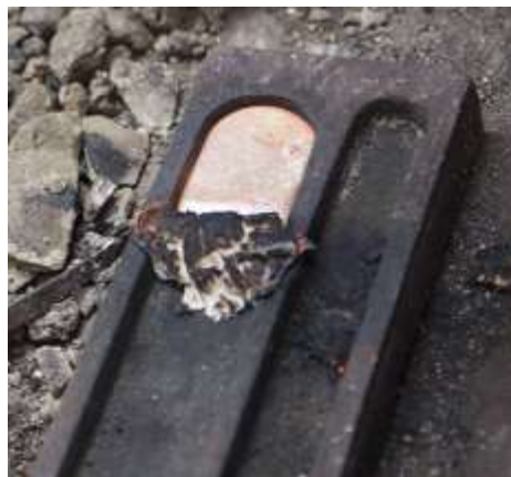
Figure 410 Mould for casting silver and gold billets © Khalid Al Busaidi
