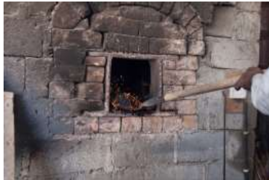
Figure 189 Cleaning out wood before preheating © Khalid Al Busaidi
