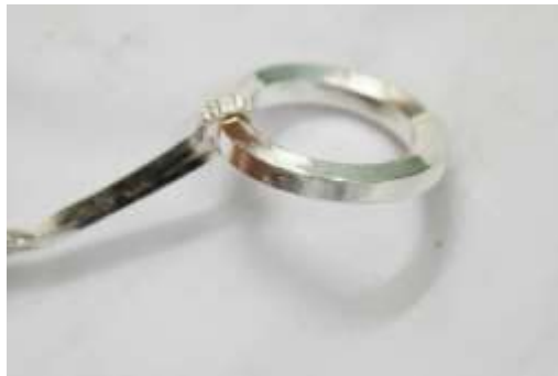
Figure 301 Attachment of rings with long rivets © Khalid Al Busaidi
