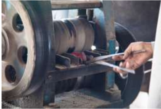
Figure 195 Roll forging the steel piece © Khalid Al Busaidi
