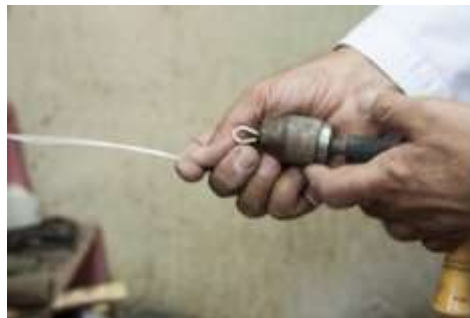
Figure 321 Attaching a wire to the hand drill © Khalid Al Busaidi
