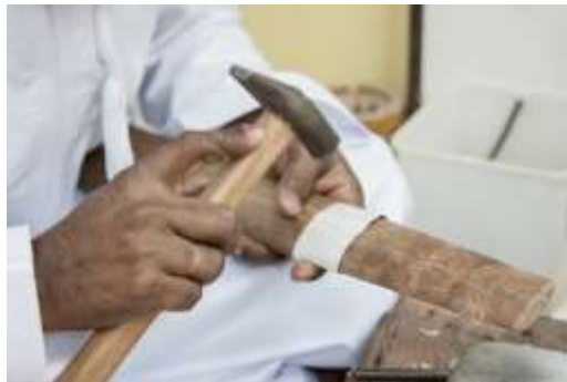
Figure 258 Forming of the scabbard upper cover to an appropriate size and shape on a former © Khalid Al Busaidi
