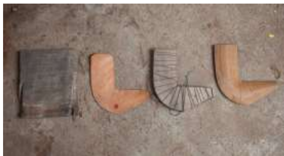
Figure 215 Elements of making wooden scabbard core © Khalid Al Busaidi
