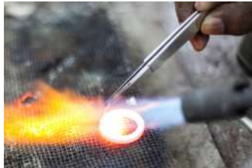
Figure 314 Soldering the ends of a ring © Khalid Al Busaidi
