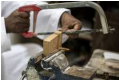
Figure 168 Clamping of the wood sample in a vice in order to cut © Khalid Al Busaidi
