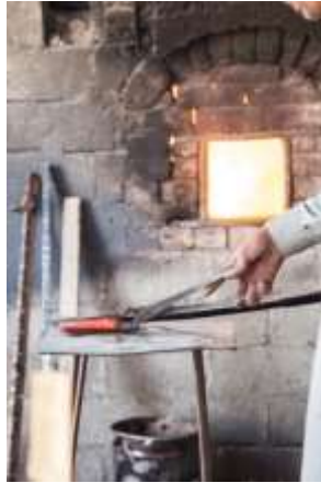
Figure 197 Removal of a partly reheated forged blade piece © Khalid Al Busaidi
