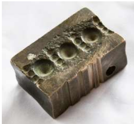
Figure 358 Small metal mould for casting silver or gold bosses © Khalid Al Busaidi
