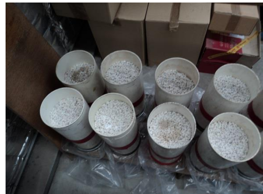
Plate 3.7 Leaching columns in position on the bench with the phosphorus fertiliser treatments applied to the surface. Note the clear plastic bag placed below each column for a collection of the leachate.
