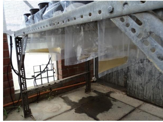
Plate 3.9 Leachate collection bags under the pots on the bench 1 of the pot experiment.
