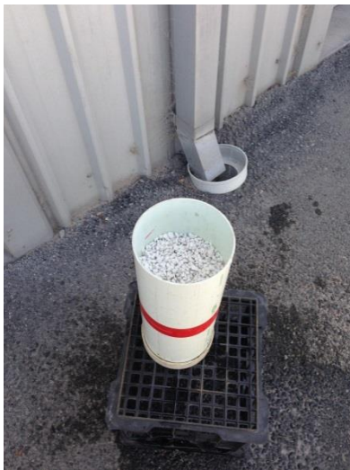
Plate 3.6 Leaching column filled with 6 L of perlite prior to the start of the experiment.
