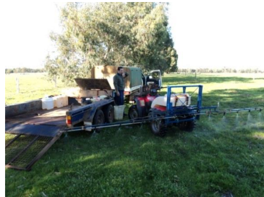
Plate 3.11 Four-wheel quad bike used for applying of liquid fertilisers, herbicides and pesticides to the field experiment sites.
